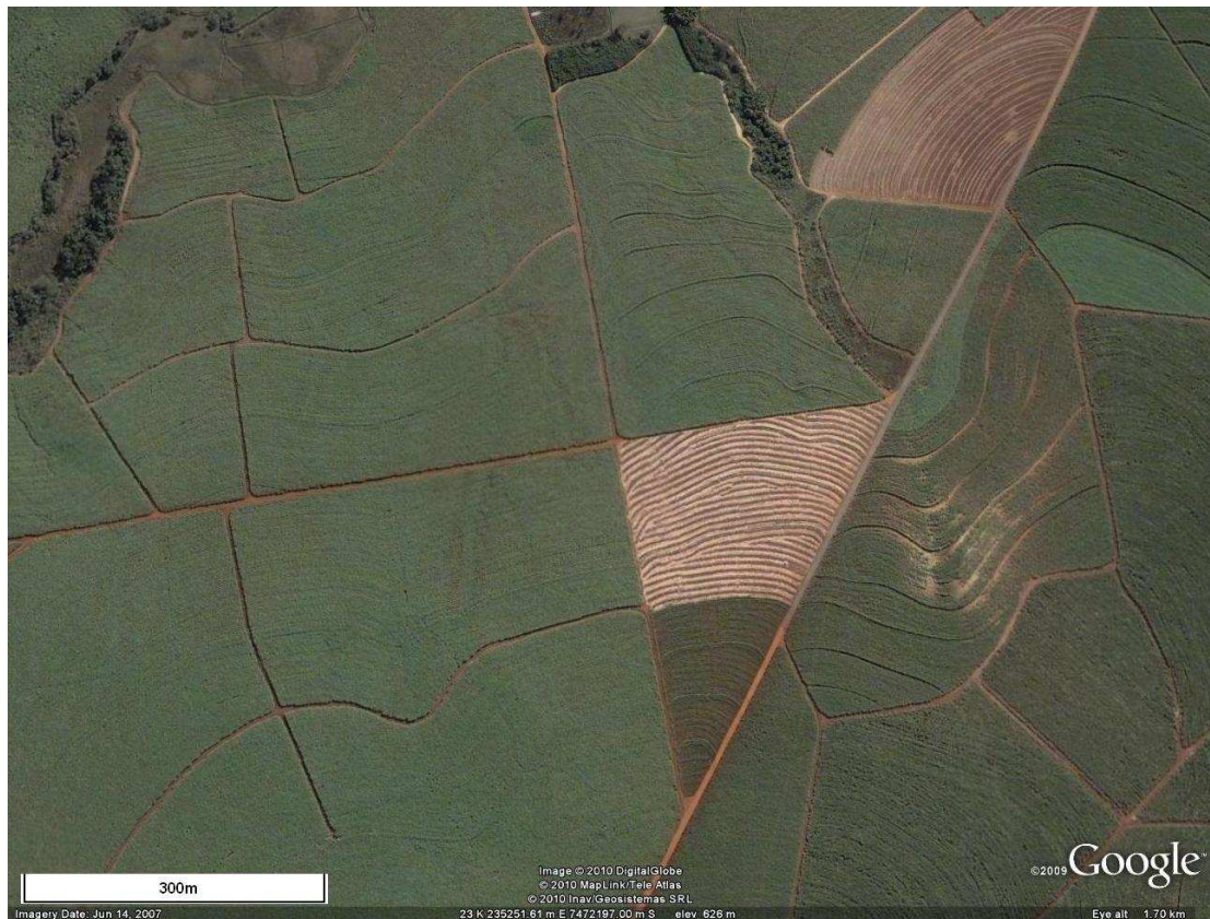
Figure 1. Example of sugar-cane established in curved patterns against slope for erosion control in Piracicaba, Brazil.
