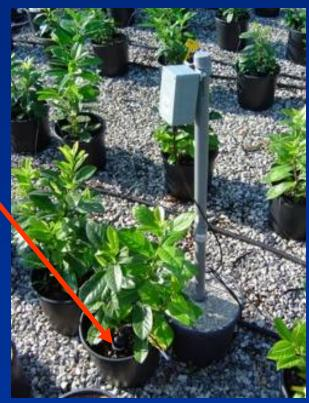
Calibration of WET-sensor for water content and pore water EC in different horticultural substrates;
