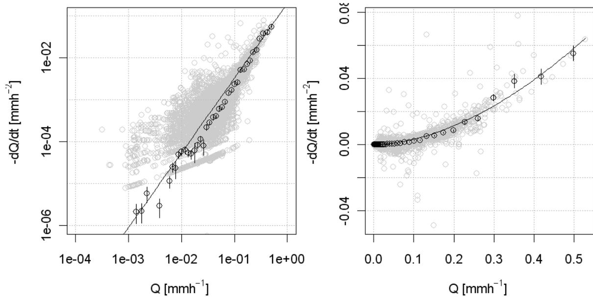
**Figure 1.** Gray: recession plot from all points with  $P=0$  and  $ET=0$  ( $\Delta t=1h$ ) on double logarithmic (left) and linear axes (right). Black: mean and standard deviation of all points in a certain bin.
