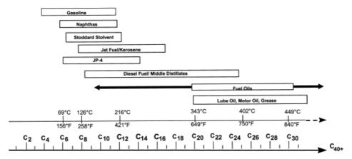
Figure 2 Approximate Carbon and Boiling Ranges of Petroleum Products [15]
