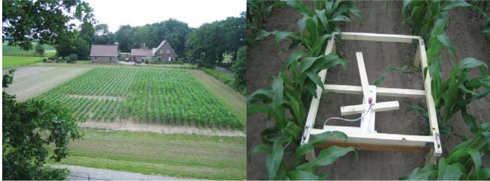
Figure 4. The field for the 2008 performance test (left) and the measurement device to measure position and orientation accuracy of the robot (right).
