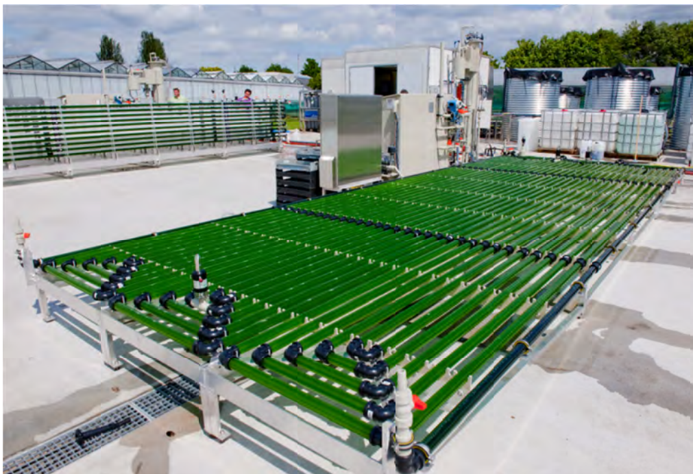
Photo 11: Overview of AlgaePARC with a horizontal tube reactor filled with algae (source Wild Frontiers/Hans Wolkers)
