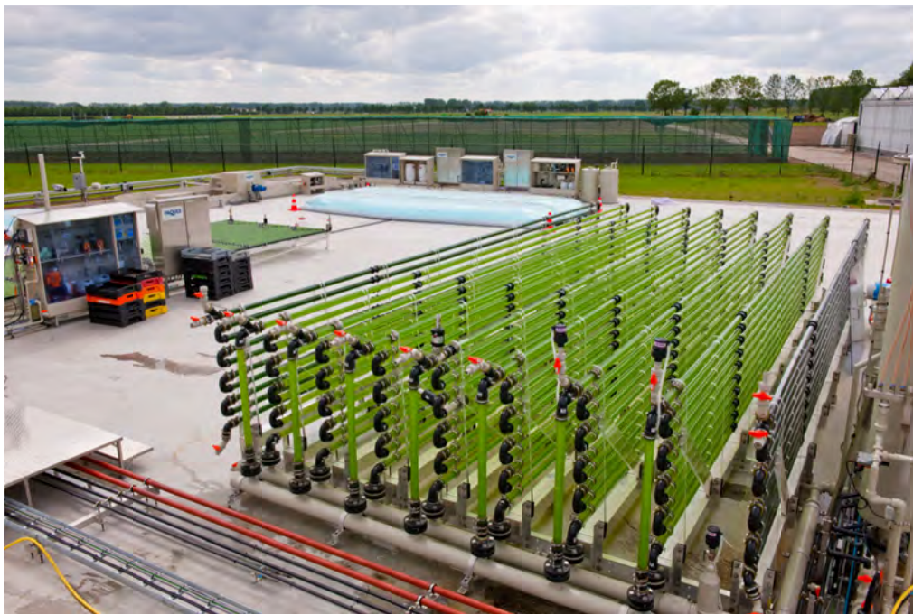
Photo 12: Three-dimensional tube reactor in AlgaePARC (source Wild Frontiers/Hans Wolkers)
