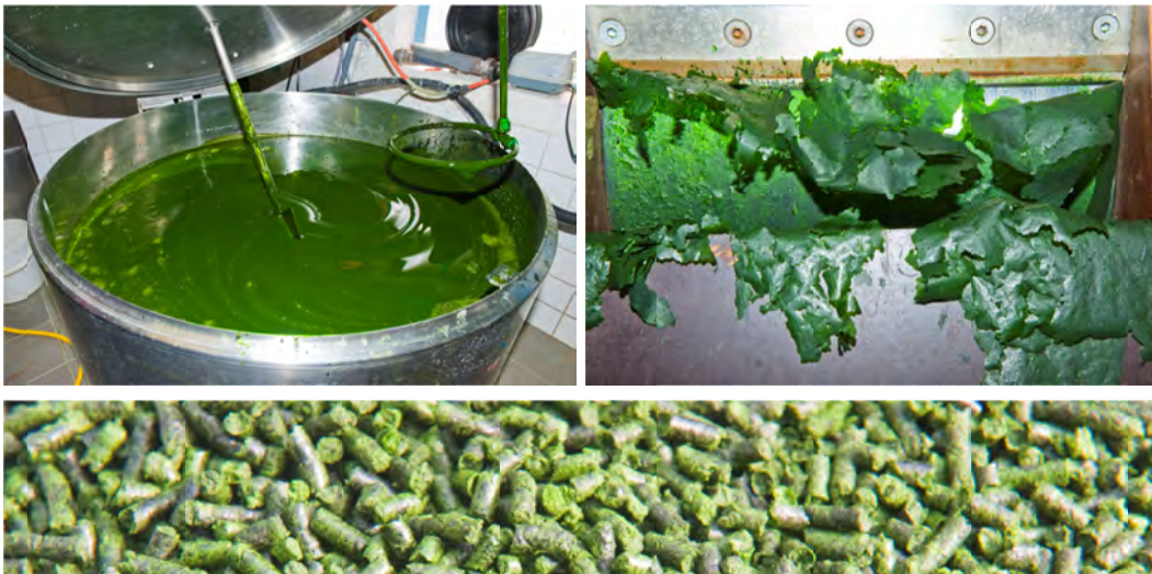
Photo 8: Highly concentrated algal soup, dried paper-thin sheets and the final product, small pellets, at Ingrepro (source Wild Frontiers/Hans Wolkers)
