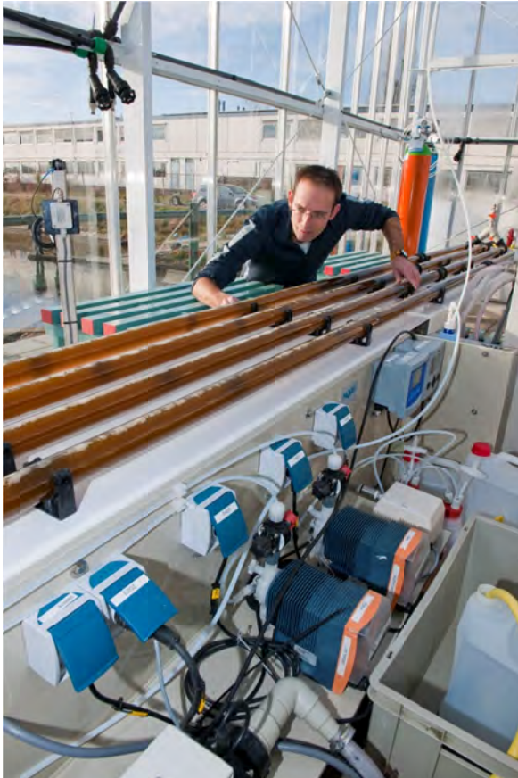
Photo 5: Algae cultivation in horizontal tube reactor at the Hogeschool Zeeland in cooperation with Wageningen University for the Zeeuwse Tong project (source Wild Frontiers/Hans Wolkers)
