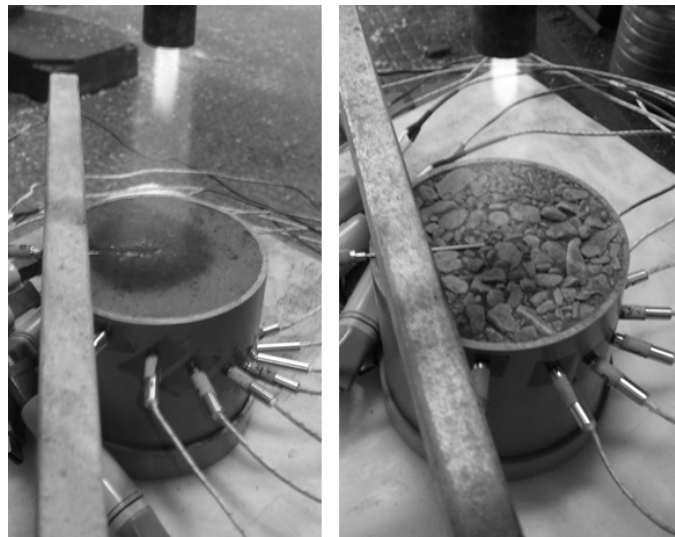
Figure 3.2 Setup of a soil column without (left) and with (right) a rock fragment cover during the burning experiment. Thermocouples were inserted in the soil column at 1-cm increments along a diagonal. The uppermost thermocouple was held in place using a metal bar.
