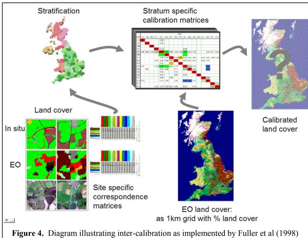
**Figure 4.** Diagram illustrating inter-calibration as implemented by Fuller et al (1998)
