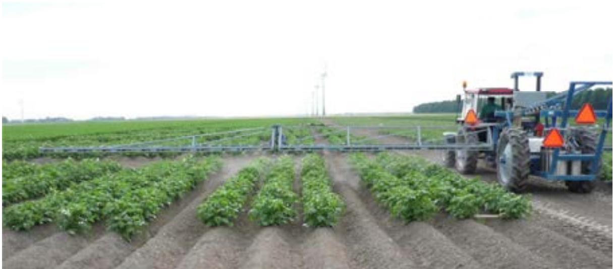
Figure 2: One of the beams of the Sosef-trial-spraying machine (in another experiment). Every time the spraying machine goes to the experimental field 10 different products can be sprayed.
