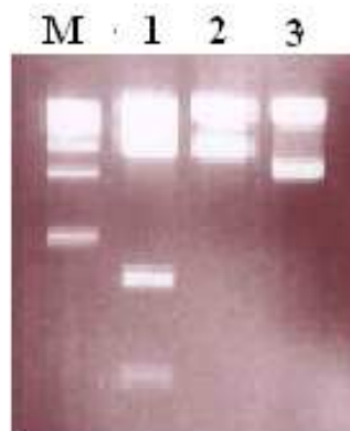
Figure 4. Digestion of 3 LR Gateway® cloned peru2 plasmids with Nhe I and Afl II restriction enzymes; M is 1kb marker; plasmid 1 gave 4 bands (2 of them less than 1 kb), plasmid 2 resulted 2 fragments but seems different from expected size, and plasmid 3 matched the expected 2 fragments (7182 and 2112 bp).
