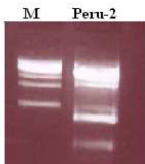
Figure 1. Peru2 plasmid digestion performed for the 2 nd time, two fragments (7182 and 2112 bp) were expected but 3 fragments (2 of them less than 1 kb) were found. We concluded the plasmid from Thomas is incorrect Peru2 plasmid; M is 1kb marker
