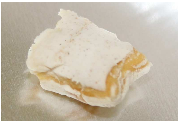
Figure 7.8: Starch, gluten, starch structure is visible after drying. Device geometry: 2.5° cone, gap 2 mm. Process conditions: 5-15 rpm, 15 min. The sample is taken from the intermediate layers of the shearing device.
