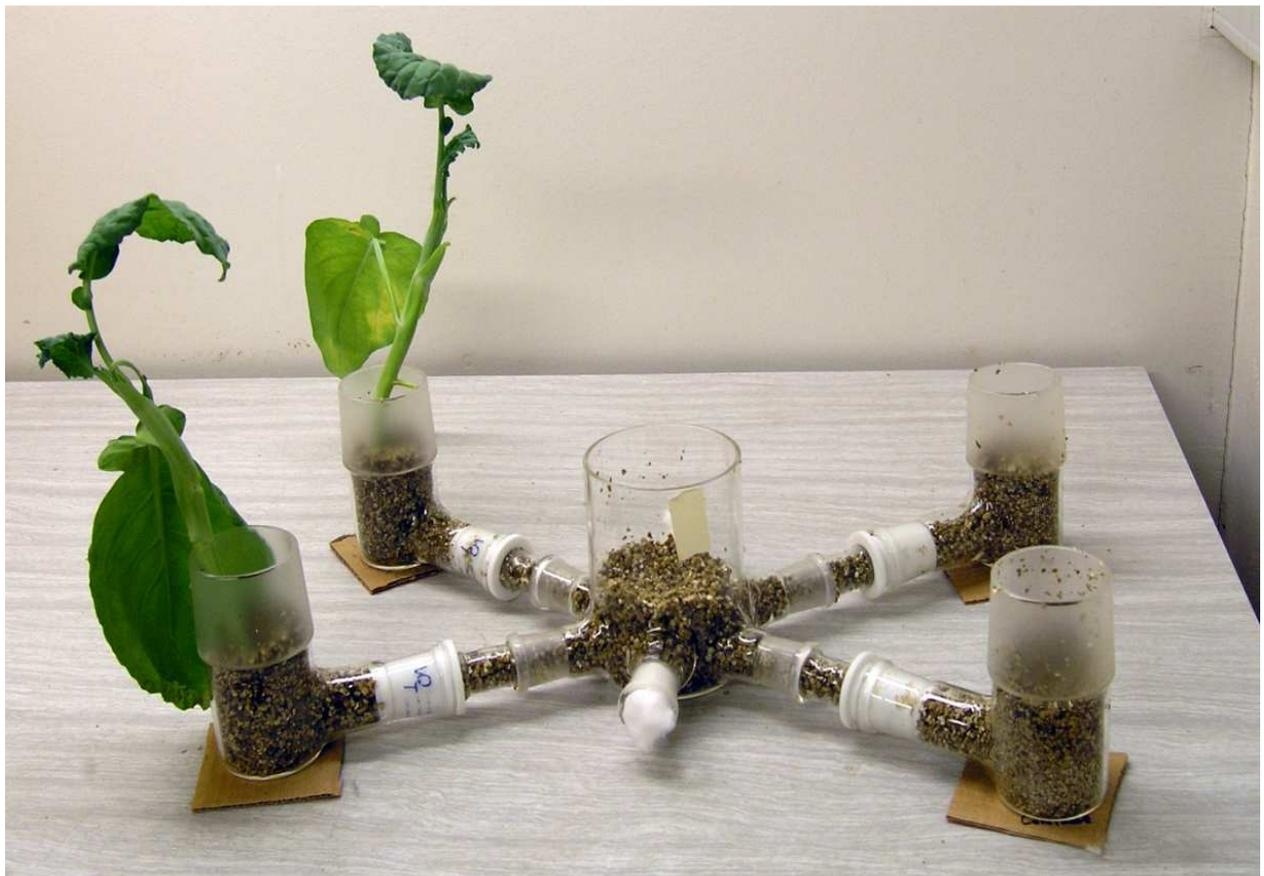
Figure 15 The four arm olfactometer running with Chinese cabbages.
