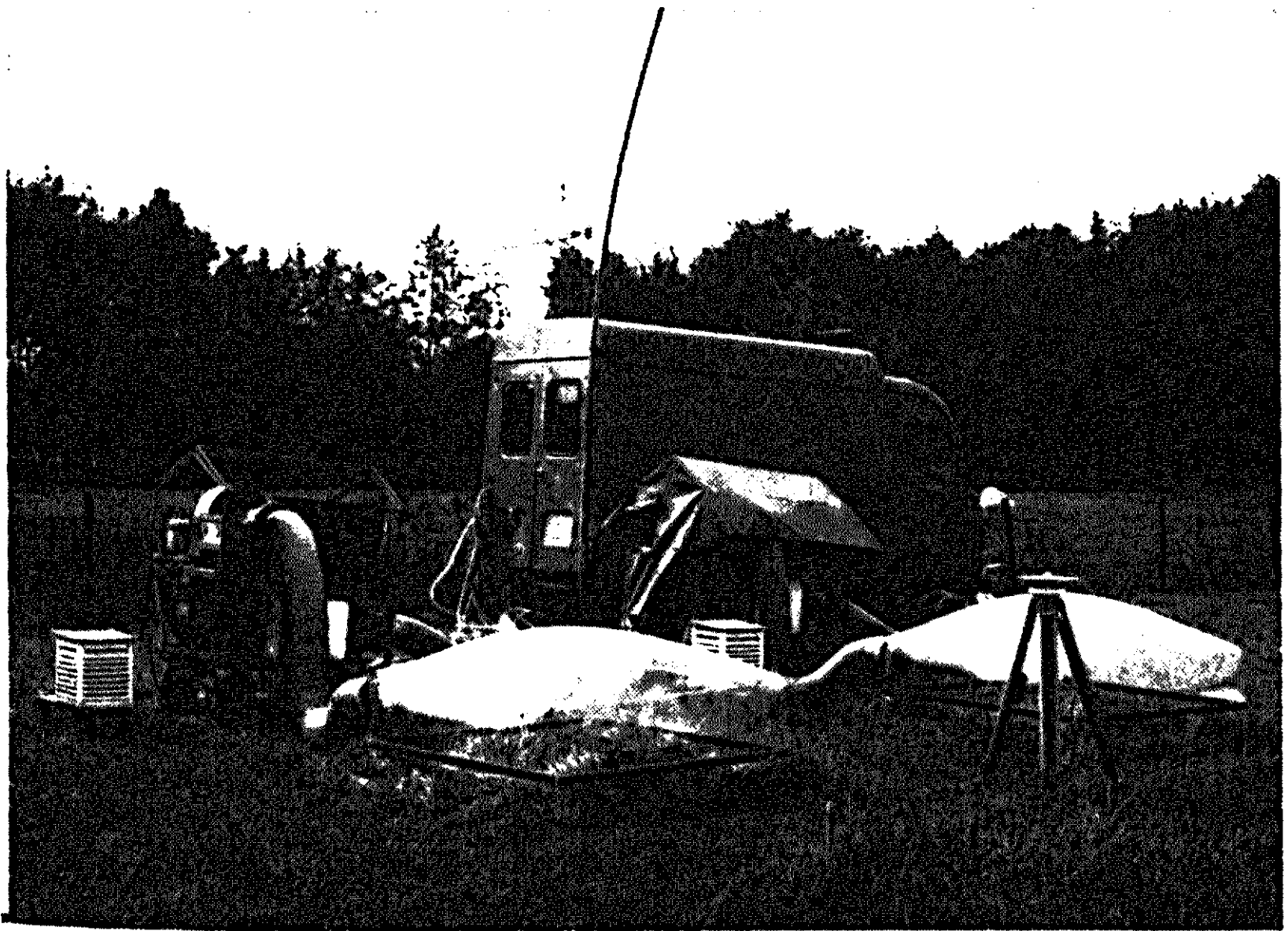
Plate 1. The mobile installation of the Centre for Agrobiological Research (Wageningen) for measuring \text{CO}_2 assimilation, respiration and transpiration of crop surfaces.
