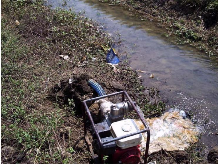
Picture 7 shows a water pump being used by farmer to pump ground water for irrigating secondary crop.
