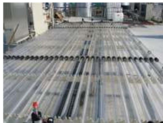
Figure 1 Horizontal tubular reactor system without algae. Location: AlgaePARC Wageningen
