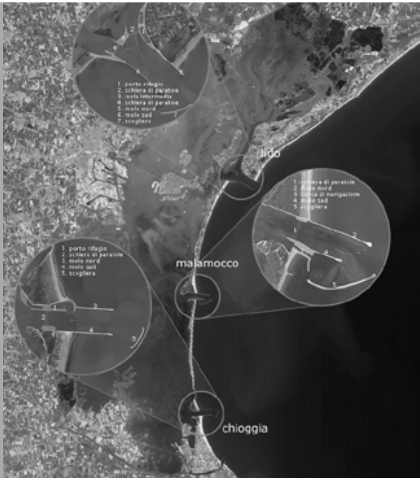
Figure 2. Project design of the mobile barrier system to protect Venice from tidal floods (MOSE) [source: Mag. Acque, 2010]
