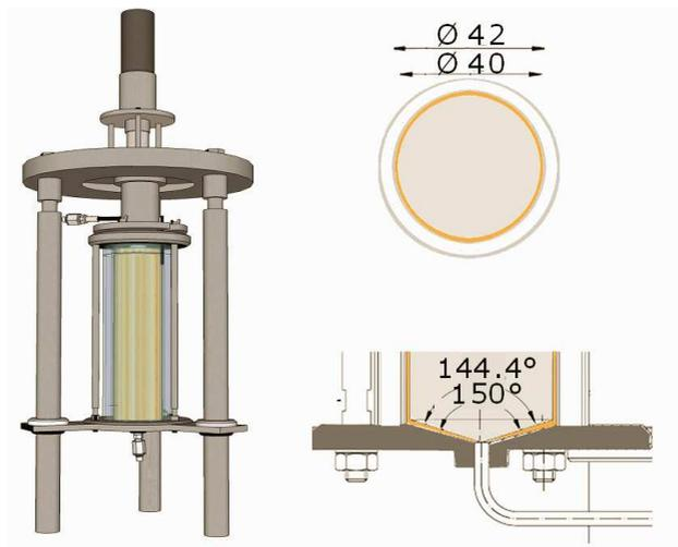
*Figure 1: Schematic drawing of the shearing device. The diameter of the rotating inner cylinder is 40 mm. The diameter of the stationary outer cylinder is 42 mm. The bottom of the shearing device is designed as a cone/plate geometry with an angle of 2.8°.*
