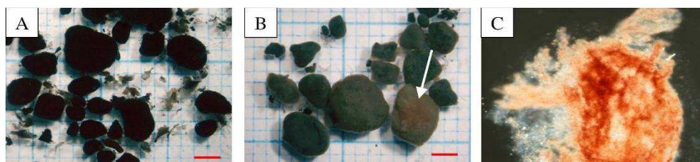
Figure 4.5 Reflected-light microscopic pictures of anaerobic sludge granules originating from R1 (A) and R2 (B) at 150 days of operation and biofilm originating from tubing of R2 (C). Bars correspond to 2 mm, arrow marks red spots of elemental selenium
