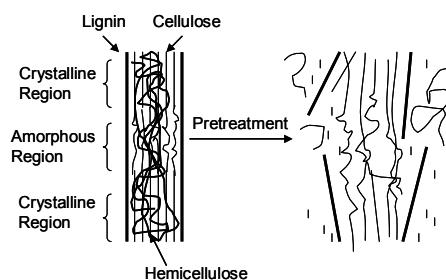
Figure 4. Effect of pretreatment on lignocellulose material (Mosier et al., 2005).
