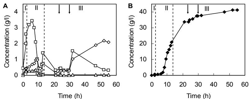
Figure 3. Profiles of glucose (□), xylose (◇), arabinose (△) (A) and lactic acid (◆) (B) in simultaneous saccharification and fermentation of lime-treated wheat straw by commercial enzyme preparation GC 220 and *Bacillus coagulans* DSM 2314. The areas between the dotted lines represent the pre-hydrolysis phase (I), the fed-batch phase (II) and the batch phase (III). Extra enzyme preparation GC220 was added at the times indicated by the arrows.
