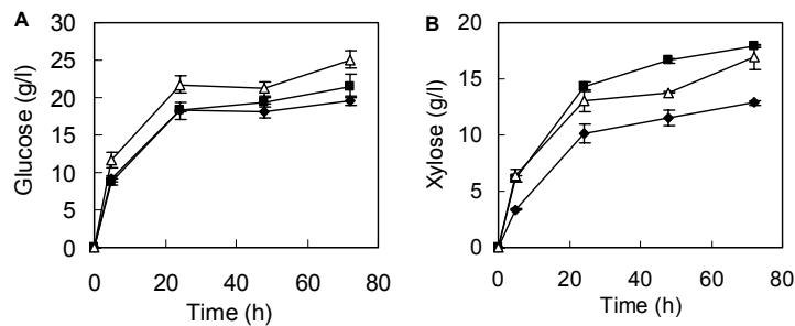
Figure 3. Influence of pH 4.0 (◆), 4.5 (■) and 5.0 (△) on the formation of glucose (A) and xylose (B) as a function of time during enzymatic hydrolysis of non-washed LTWS (169.1 mg enzyme preparation per g DM LTWS, 50°C). The error bars in symbols denote deviation of duplicate experiments.
