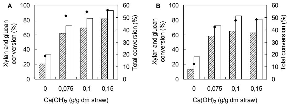
Figure 1. Effect of  $\text{Ca(OH)}_2$  loading rate (g/g dm straw) on enzymatic hydrolysis of xylan to xylose (▨) and glucan to glucose (□) in lime pretreated wheat straw (washed insoluble fraction). Enzyme loading rate was 116 IFPU/g dm for GC 220 (A) and 56 IFPU/g dm for Cellubrix (B). Incubation was at 40°C, for 24h, and pH was buffered at 5.0. The total conversion (◆) is expressed as total dry matter solubilized after pretreatment and enzymatic hydrolysis.
