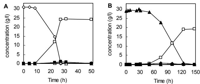
Figure 1. Typical conversion of (A) glucose ( $\diamond$ ) and (B) xylose ( $\blacktriangle$ ) into L(+)-lactic acid ( $\square$ ) by *R. oryzae* CBS 127.08. The by-products were xylitol ( $\blacklozenge$ ), glycerol ( $\triangle$ ) and ethanol ( $\blacksquare$ ).
