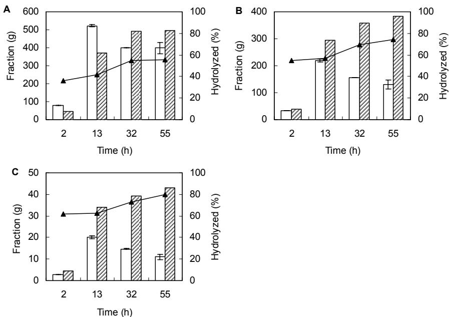
Figure 4. Insoluble fraction (□) and hydrolyzed soluble fraction (▨) (g) (calculated by the difference between initial amounts and analyzed insoluble amounts) of the polysaccharide glucan (A), xylan (B) and arabinan (C) at various time points during the simultaneous saccharification and fermentation of lime-treated wheat straw. Figure represents also the percentage of polysaccharide hydrolyzed into soluble products (▲). The error bars denote the deviation of duplicate analysis.
