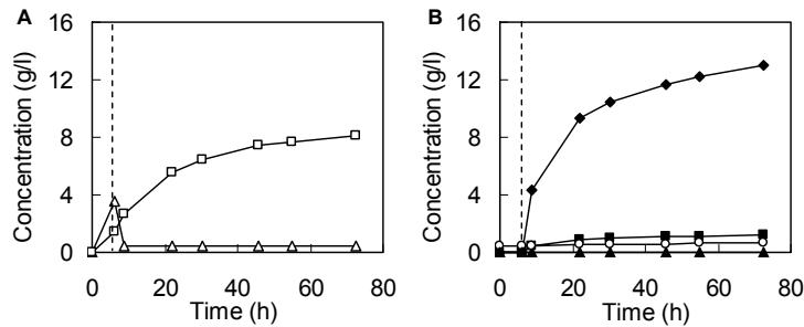
Figure 9. SSF of washed LTWS at pH 5.0 in the presence of PenStrep with formation of glucose ( $\Delta$ ), xylose ( $\square$ ) and ethanol ( $\blacklozenge$ ) (A) and glycerol ( $\blacksquare$ ), acetic acid ( $\circ$ ) and lactic acid ( $\blacktriangle$ ) (B). Dotted lines represent the end of pre-hydrolysis and moment of yeast addition.
