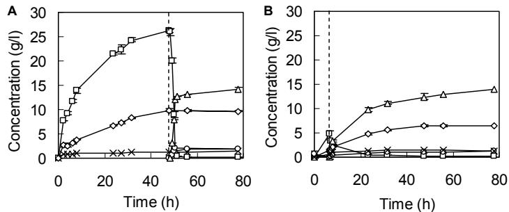
Figure 10. Comparison of SHF (hydrolysis at 50°C and fermentation at 37°C) (A) and SSF (pre-hydrolysis at 50°C and SSF at 37°C) (B) of washed LTWS in the presence of PenStrep with the formation of saccharification products glucose (□), xylose (◇) and arabinose (×) and fermentation products, ethanol (△) and glycerol (○) by *S. cerevisiae*. Dotted lines represent moment of yeast addition. The error bars in symbols denote deviation of triplicate experiments.
