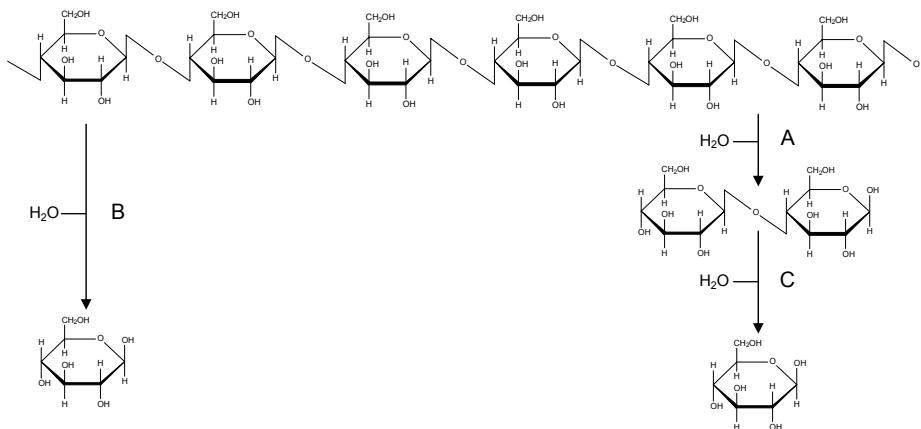
Figure 5. Schematic representation of enzymatic hydrolysis of cellulose to cellobiose by endoglucanase (A) and to glucose by exoglucanase (B). Cellobiose can be hydrolysed to glucose by  $\beta$ -glucosidase (C).
