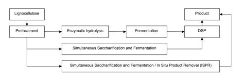
Figure 10. Schematic overview of lignocellulose-to-product process including the SHF and SSF approach.
