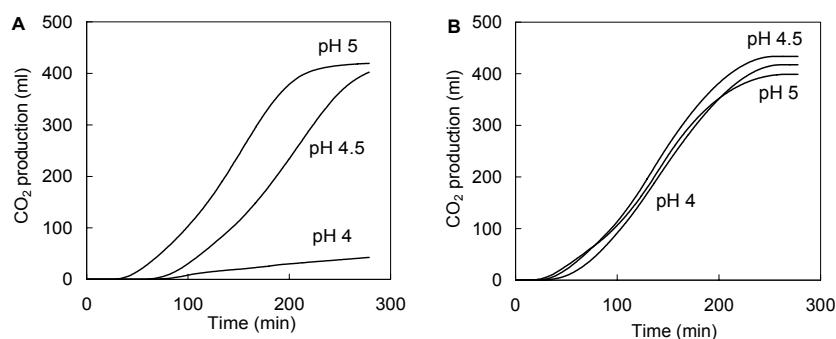
Figure 7. Production of CO<sub>2</sub> (as equimolar of ethanol) during fermentation of unwashed (A) and washed (B) lime-pretreated wheat straw by *S. cerevisiae* at 32°C and pH 4, 4.5 and 5.
