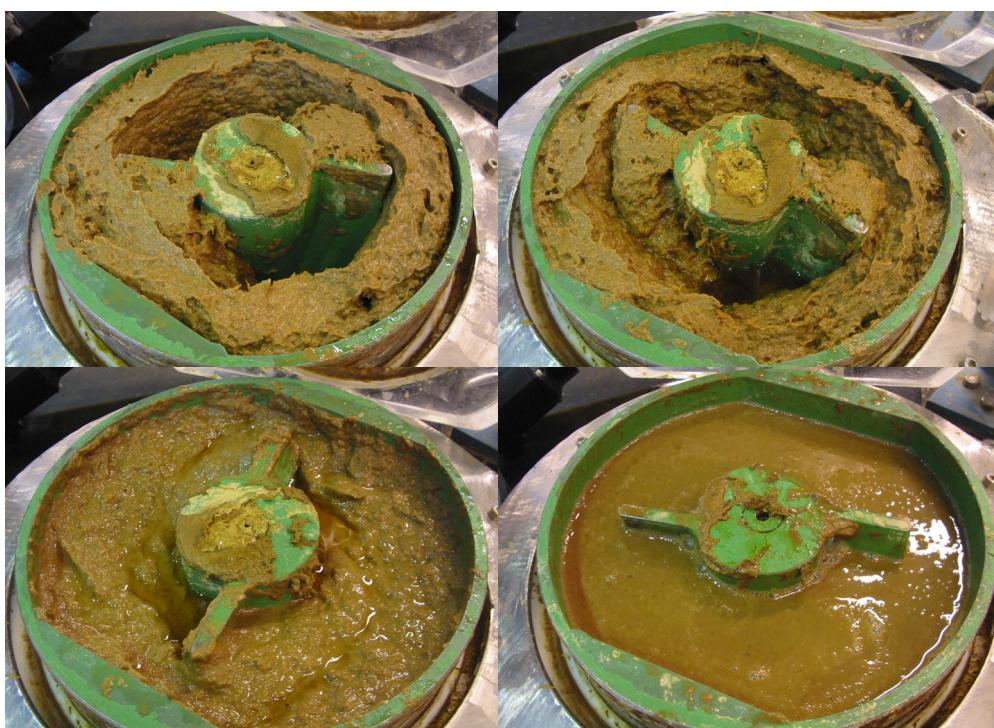
*Figure 3.* View of bench-scale hydrolysis of lime pretreated wheat straw during enzymatic hydrolysis at  $t = 0$  (top left), 0.5 (top right), 2 (bottom left) and 24 h (bottom right) after adding enzymes
