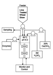
Figure 1. Schematic representation of the simultaneous saccharification and fermentation of lime-treated wheat straw to lactic acid.
