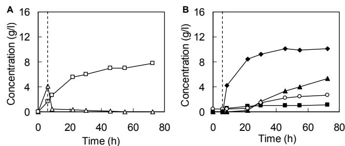
Figure 8. Typical SSF of washed LTWS at pH 5.0 with formation of glucose (△), xylose (□) (A) and ethanol (◆), glycerol (■), acetic acid (○) and lactic acid (▲) (B). Dotted lines represent the end of pre-hydrolysis and moment of yeast addition.
