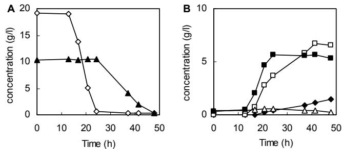
Figure 4. Fermentation of mild-temperature alkaline-treated wheat straw hydrolysate by *R. oryzae* CBS 112.07 (A) Substrate consumption of glucose (◊) and xylose (▲). (B) Product formation of lactic acid (□), xylitol (◆), glycerol (△) and ethanol (■).
