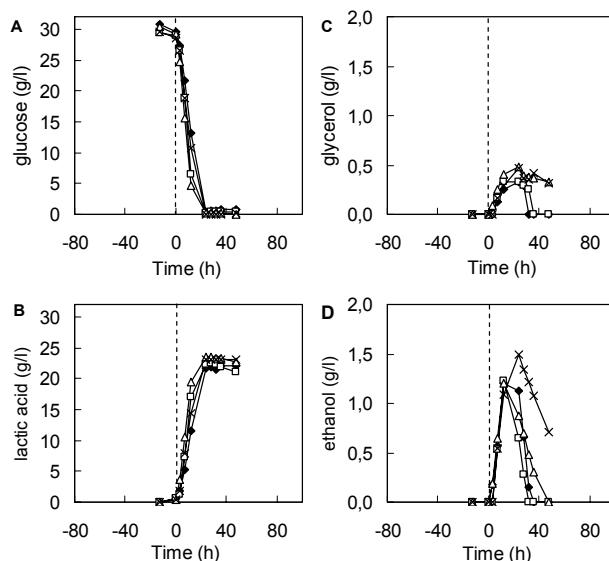
Figure 5. Effect of different medium volumes (aeration rates) on the conversion of glucose (A) by *R. oryzae* CBS 112.07 to lactic acid (B), glycerol (C) and ethanol (D) in 250-ml baffled shake flasks with medium volumes of 75 (◆), 100 (□), 125 (△) and 150 ml (x). Dotted lines represent the start of detectable consumption of glucose.
