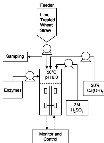
Figure 1. Schematic representation of the simultaneous saccharification and fermentation of lime-treated wheat straw to lactic acid.
