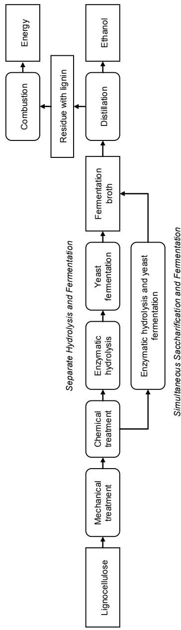
Figure 1. Schematic overview of the lignocellulose-to-ethanol process by separate hydrolysis and fermentation (SHF) and simultaneous saccharification and fermentation (SSF) routes. In the scope of this study, the focus was on the enzymatic hydrolysis and yeast fermentation steps.
