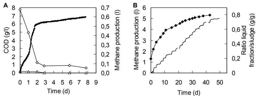
Figure 2. (A) Dissolved chemical oxygen demand (COD) ( $\diamond$ ), dissolved volatile fatty acids (VFA-COD) ( $\triangle$ ) and methane production (line) during the anaerobic biodegradability test with ten times diluted liquid fraction (20 ml in total of 200 ml). Data were corrected for the blank. (B) Methane production (line) during the accumulation test where the ratio liquid fraction per sludge ( $\blacklozenge$ ) is increased. All data are represented as averages of duplicate experiments.
