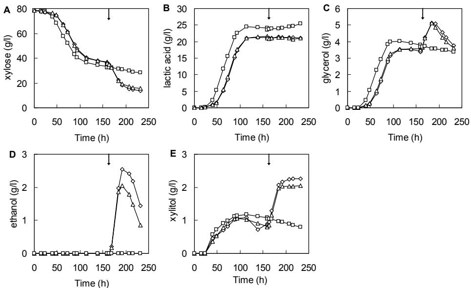
Figure 1. Conversion of xylose (A) by *R. oryzae* CBS 112.07 to lactic acid (B), glycerol (C), ethanol (D) and xylitol (E). The arrow represent the moment of an extra addition of  $(\text{NH}_4)_2\text{SO}_4$  ( $\diamond$ ),  $(\text{NH}_4)_2\text{PO}_4$  ( $\triangle$ ) and blank with demi water ( $\square$ ).
