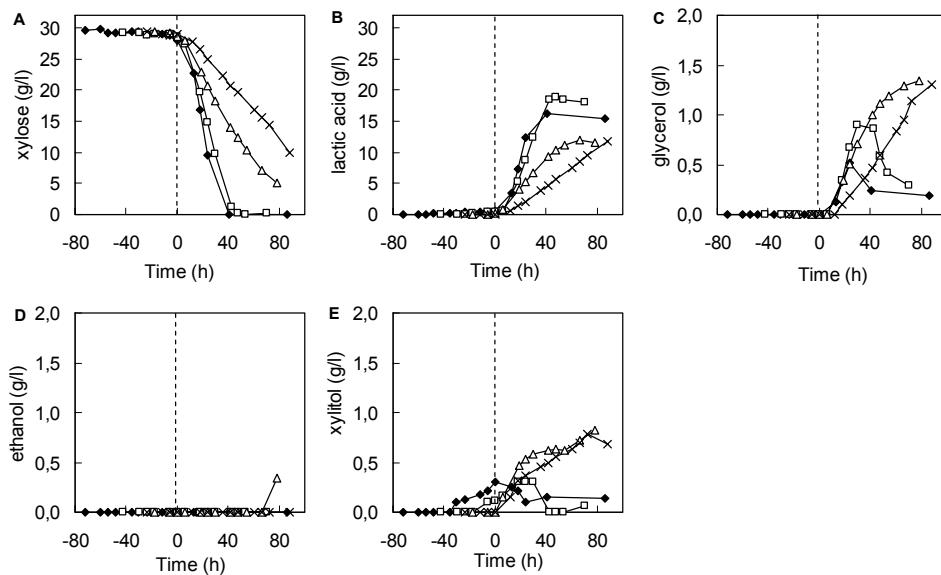
Figure 4. Effect of different medium volumes (aeration rates) on the conversion of xylose (A) by *R. oryzae* CBS 112.07 to lactic acid (B), glycerol (C), ethanol (D) and xylitol (E) in 250-ml baffled shake flasks with medium volumes of 75 (●), 100 (□), 125 (△) and 150 ml (×). Dotted lines represent the start of detectable consumption of xylose.
