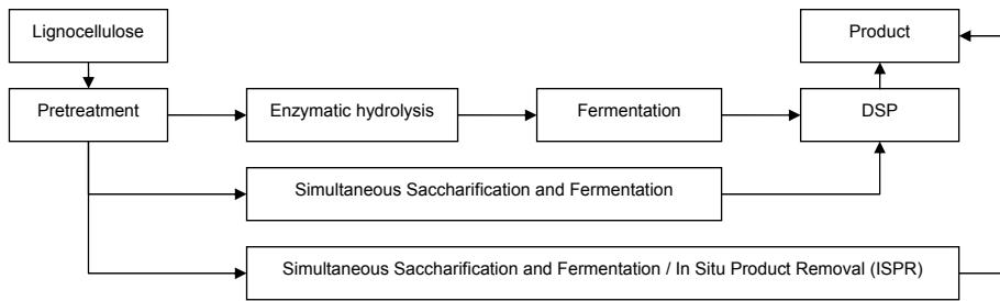
Figure 10. Schematic overview of lignocellulose-to-product process including the SHF and SSF approach.
