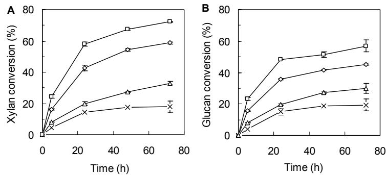
Figure 2. Conversion of xylan to xylose (A) and glucan to glucose (B) in lime-treated (0.1 g/g) wheat straw with GC 220 and dosage of 2.1 (x), 4.1 (Δ), 8.2 (◊) and 16.3 (□) IFPU/g dm straw at pH 4.5 and 50°C.
