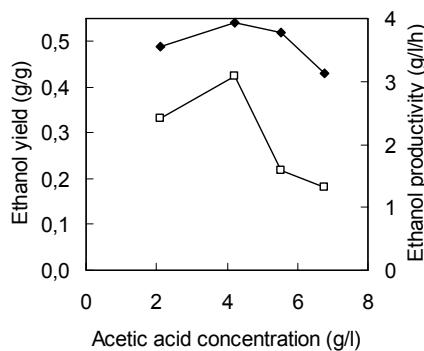
Figure 6. Effect of acetic acid concentration in lime-pretreated straw on ethanol yield (◆) and productivity (□) by *S. cerevisiae* fermented at pH 5 and 32°C.
