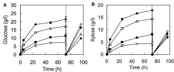
Figure 4. Influence of enzyme concentration of 21.1 (◇) 42.3 (■) 84.6 (△) 169.1 (◆) mg per g DM on the formation of glucose (A) and xylose (B) as a function of time during enzymatic hydrolysis of non-washed LTWS (pH 4.5, 50°C). The dotted lines represent the “re-start” hydrolysis of washed residue with 169.1 mg enzyme preparation per g DM LTWS. The error bars in symbols denote deviation of duplicate experiments.
