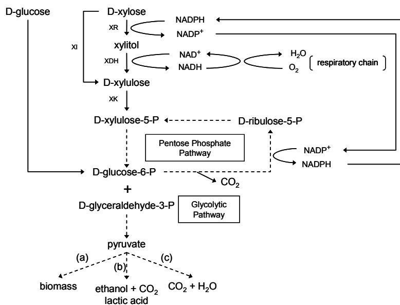
Figure 3. Proposed pathways for the catabolism of xylose, adapted from Schneider (1989). XI, xylose isomerase; XR, xylose reductase; XDH, xylitol dehydrogenase; XK, xylulose kinase. Pyruvate functions as substrate for growth (a), fermentation (b) and/or respiration (c).
