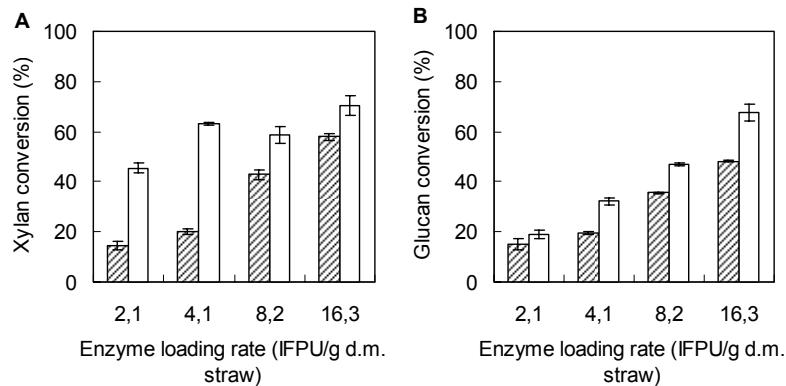
Figure 4. Effect of enzyme loading rate on xylan (A) and glucan (B) conversion from lime-treated wheat straw. Bars indicate conversion based on monomeric sugars in supernatants after enzymatic hydrolysis (▨), and monomeric sugars after supernatants were treated with 1 M sulphuric acid (□). Enzymatic incubation for 24 h with GC 220 at pH 4.5 and 50°C. Error bars represent minimum and maximum values
