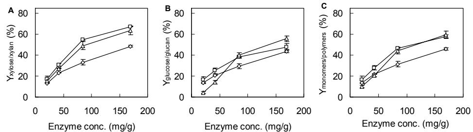
Figure 2. Effect of enzyme concentration at pH 4.0 ( $\diamond$ ), 4.5 ( $\square$ ) and 5.0 ( $\triangle$ ) on the hydrolysis yield of xylan to xylose (A) and yield of glucan to glucose (B) in non-washed LTWS (72 h, 50°C). Figure C represents the overall yield of xylose and glucose (%) formed from xylan and glucan. The error bars in symbols denote deviation of duplicate experiments.
