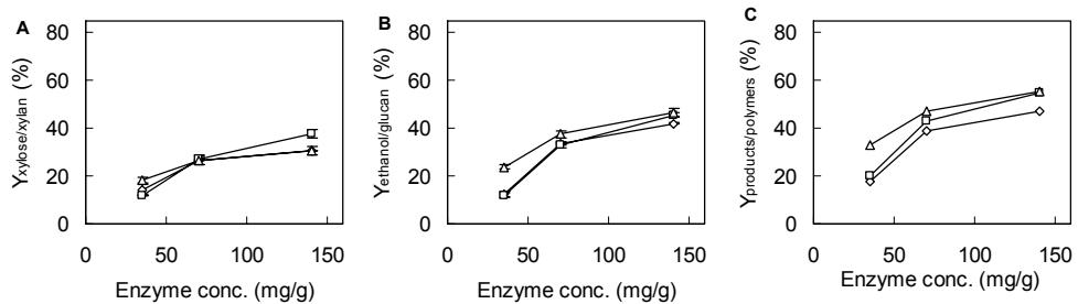
Figure 7. Effect of enzyme concentration at pH 4.0 (◇), 4.5 (□) and 5.0 (△) on the SSF of xylan-to-xylose (A) and glucan via glucose to ethanol (B) in washed LTWS (72 h). Figure C represents the overall conversion of xylan and glucan to remaining glucose and xylose and to ethanol, carbon dioxide, glycerol, acetic acid and lactic acid. The error bars in symbols denote deviation of duplicate experiments.
