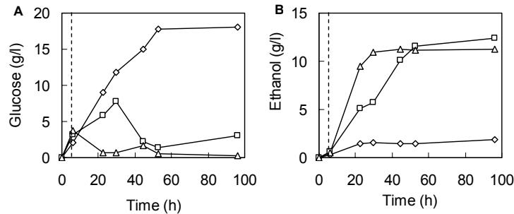
Figure 5. Formation of glucose (A) and ethanol (B) by *S. cerevisiae* during SSF of non-washed LTWS at pH 4.0 (◊), 4.5 (□) and 5.0 (△). Dotted lines represent the end of pre-hydrolysis and moment of yeast addition.
