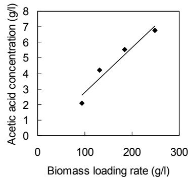
Figure 5. Acetic acid concentration in lime-pretreated wheat straw, as a function of dry matter loading rate (lime pretreatment conducted at 0.1 g/g on dry biomass basis).
