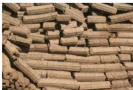
Figure 8.1: Jatropha seedcake briquettes to be used as fuel (pic J. van Eijck)
