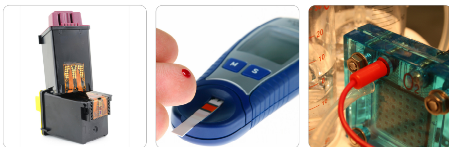
Figure 1.1 Illustrations of microfluidic devices: ink-cartridges (left), portable blood sugar monitor (center), and hydrogen fuel cell (right).
