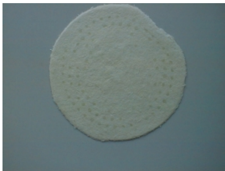
Figure 3.5: Pulp pad after enzymatic treatment
