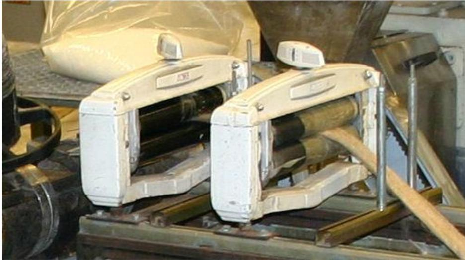
Figure-3: Jute sliver feeder
