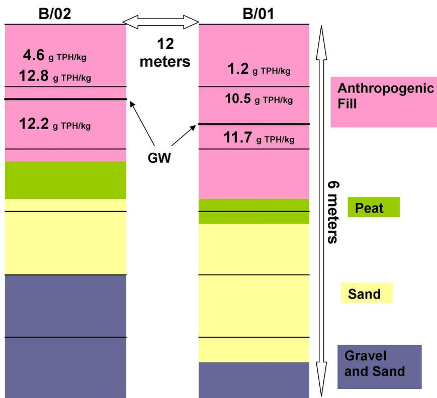
Figure 3. Lithology within source zone at the location of piezometers B/01 and B/02.
