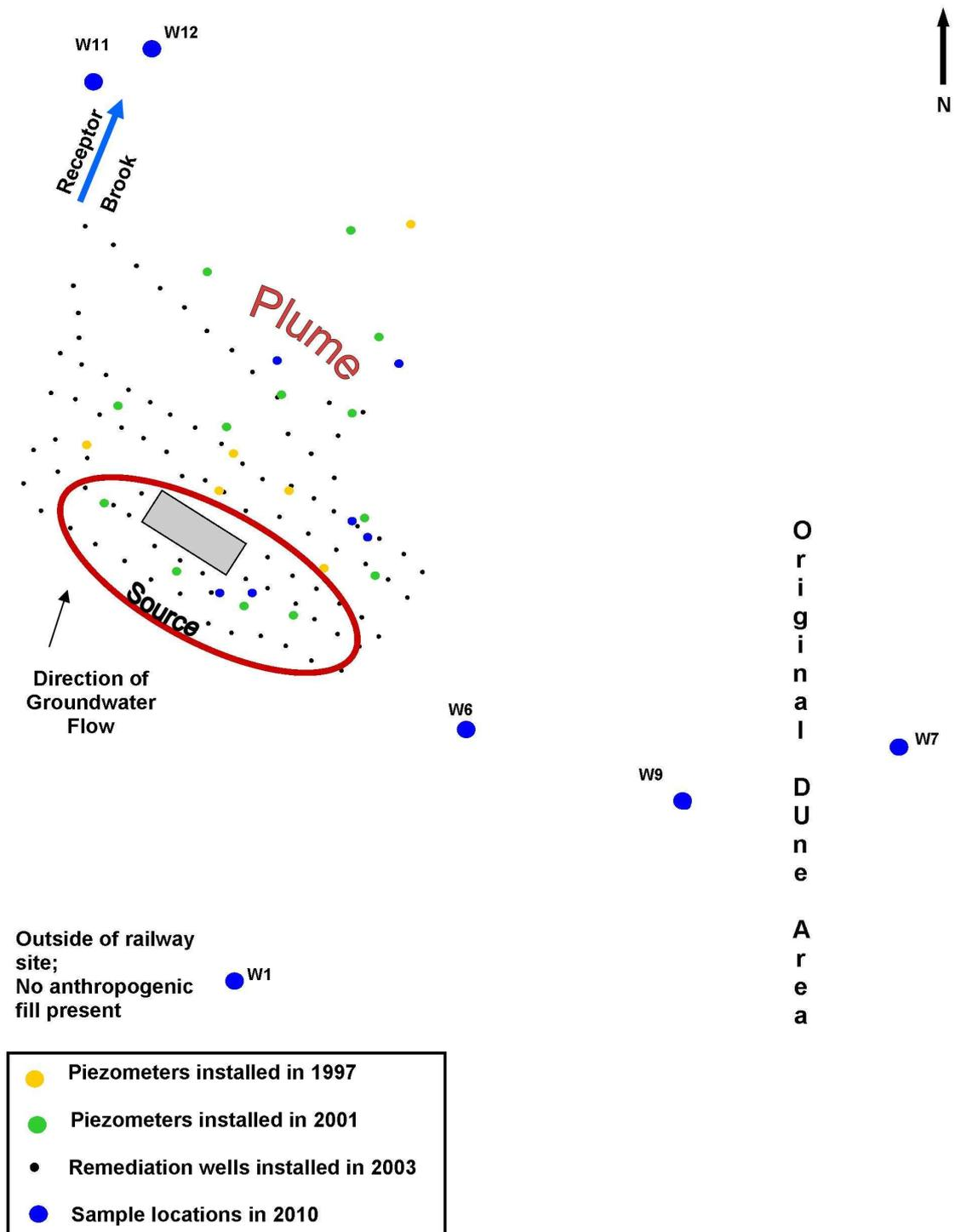
Figure 2. General overview of Węgliń, Poland contaminated railway site which shows the relationship between existing piezometers and the outermost sampling locations.
