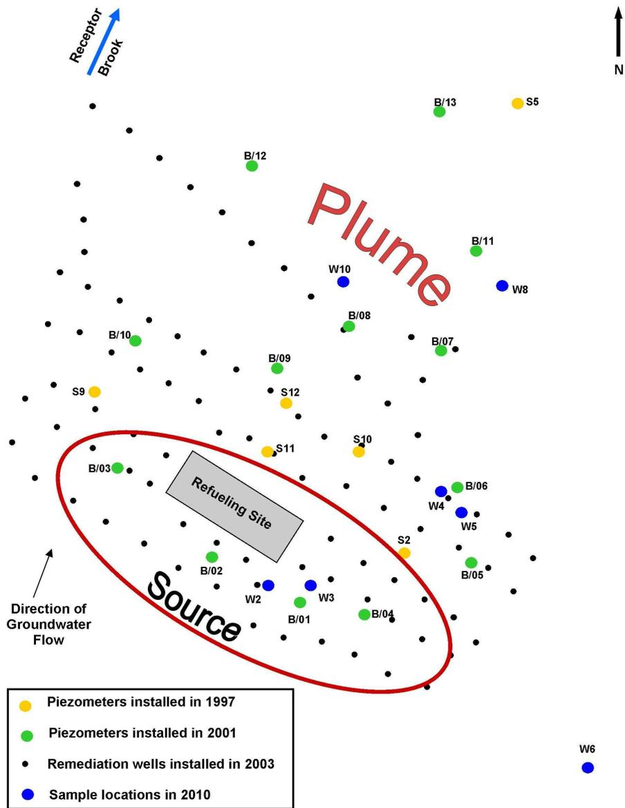
Figure 1. Węgliniec, Poland contaminated railway site, including existing piezometers, remediation wells, and sampling locations in the center of the site.
