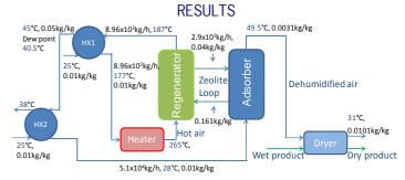
Simultaneous optimization gives opportunities for latent heat recovery through heat exchanger HX2: Overall efficiency 113%. Simultaneously optimized conventional dryer 54% efficient
