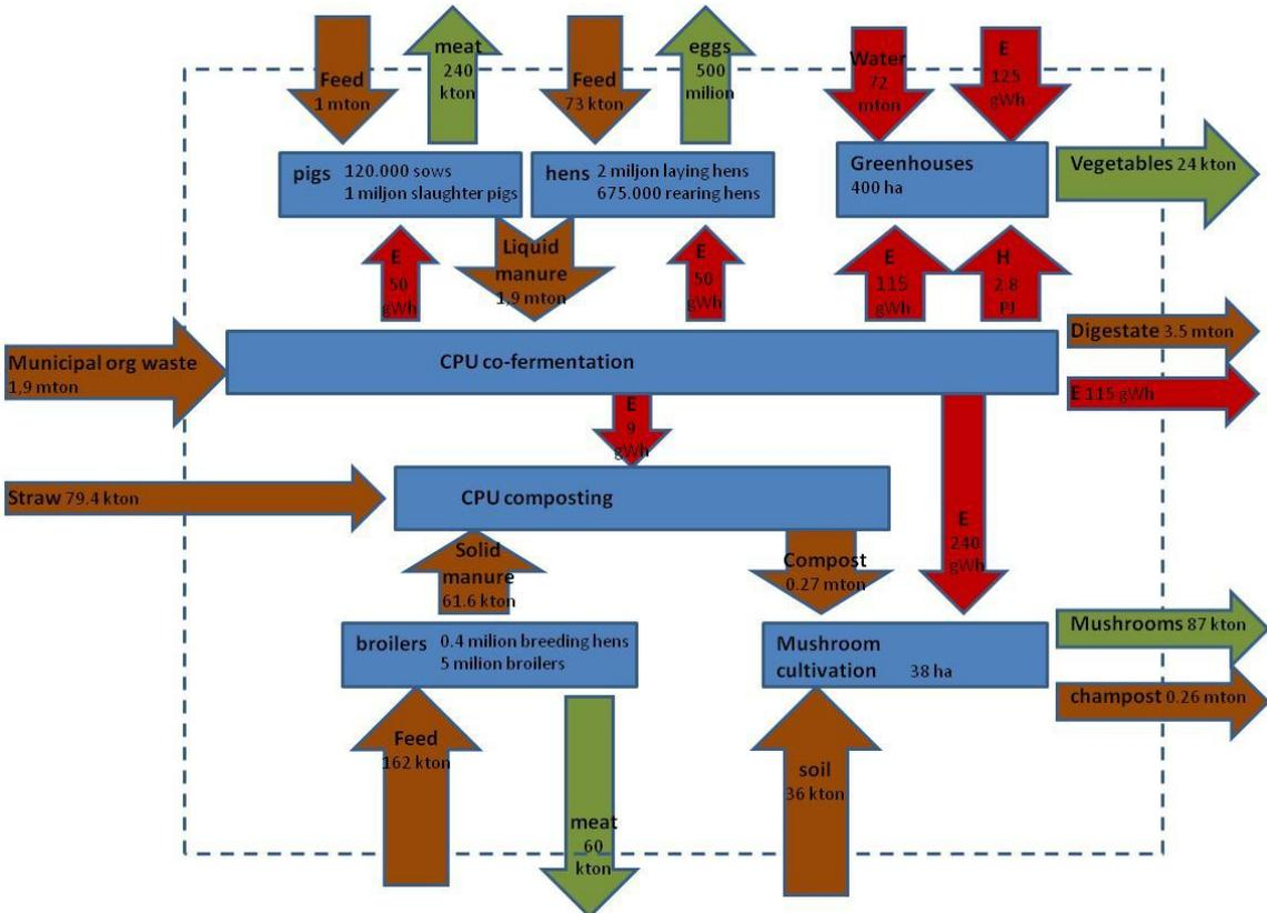
Figure 1.1. A schematic overview of the internal product and energy flows of Greenport Shanghai, the input needed for the different processes (brown arrows aimed inside) and output of food products (green arrows aimed outside) and non food products (brown arrows aimed outside) E = electricity, H = heat.
