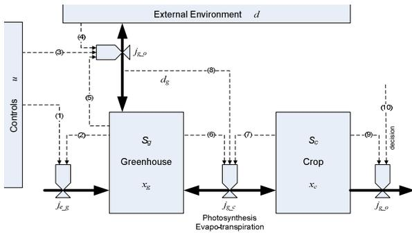
Fig. 1. Mass and energy fluxes in greenhouse system (solid lines) and information flows (dashed lines).
