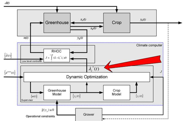
Fig. 4. Integrated optimal control. Transfer of strategic information via crop co-states. Receding horizon optimal control on the operational level, using the same economic goal function plus weather forecast.
