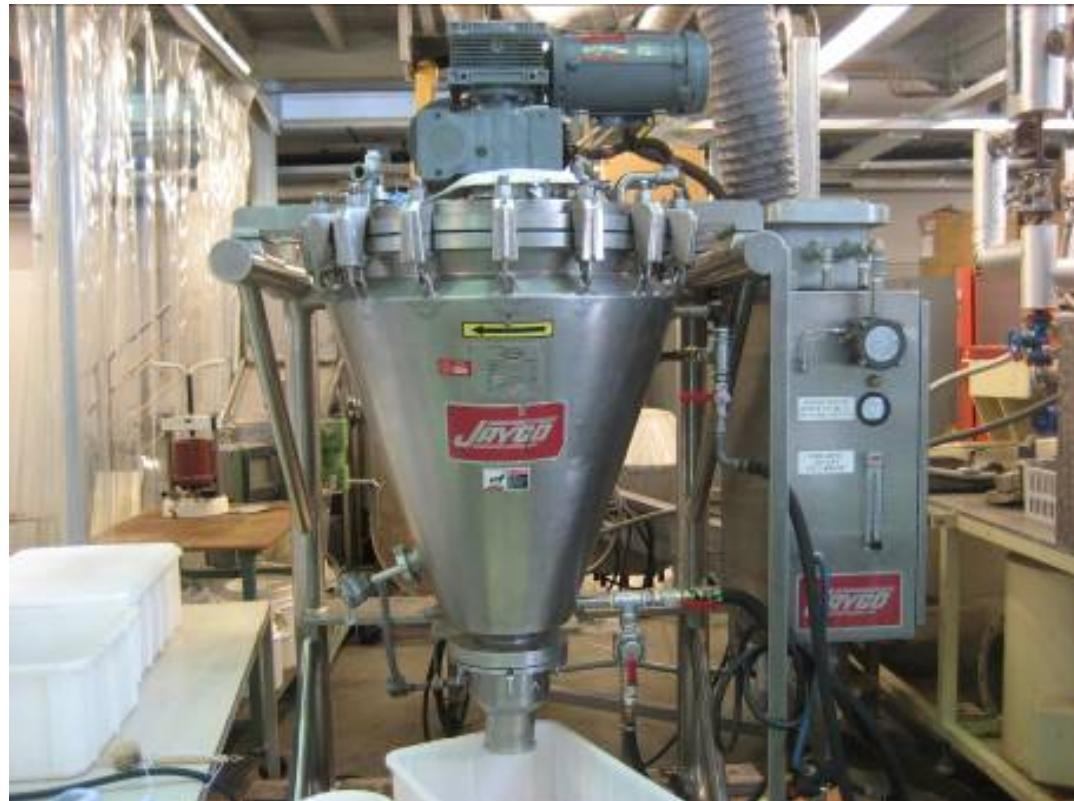
*High solids, conical screw reactor*
