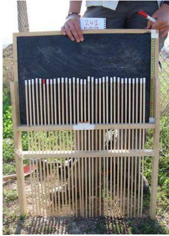
Fig 2.3: Pin meter for measurements of Random Roughness
