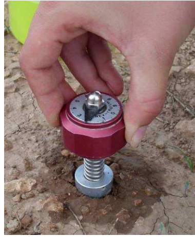
Fig 2.4: Pocket vane tester for cohesion measurements
