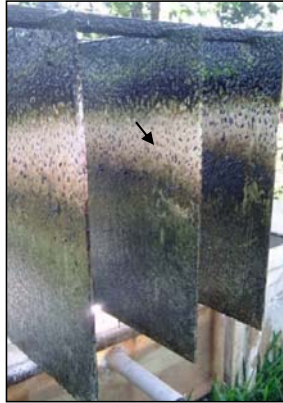
Figure 2.8: Baffles of pond 2 during period 1, note the dislodging of biofilm by Chironomidae larvae as shown by the arrow
