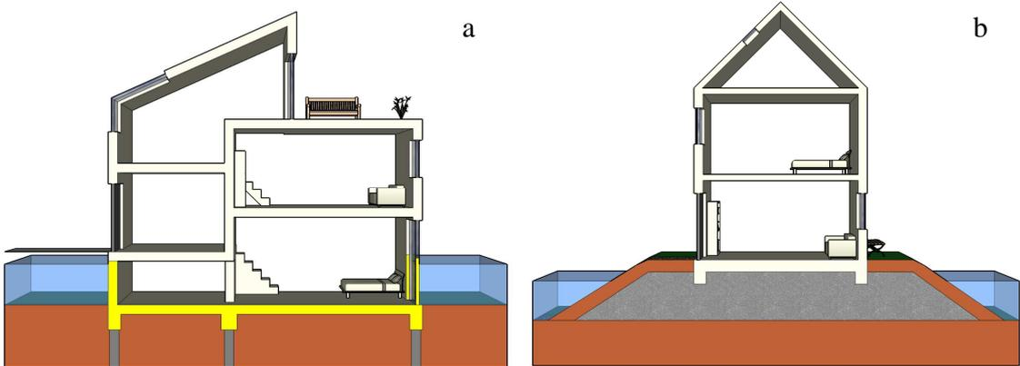
Figure 4. Flood proof house with glass walls (a) and Flood proof house on a dike or elevated area (b) (Xplorelab, 2008).
