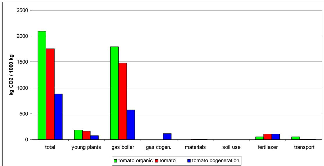
Figure 2: Tomato crop: total and components of the CO<sub>2</sub> emission (kg CO<sub>2</sub>/ ton) of an organic crop and a regular crop with and without heating with a cogeneration.
