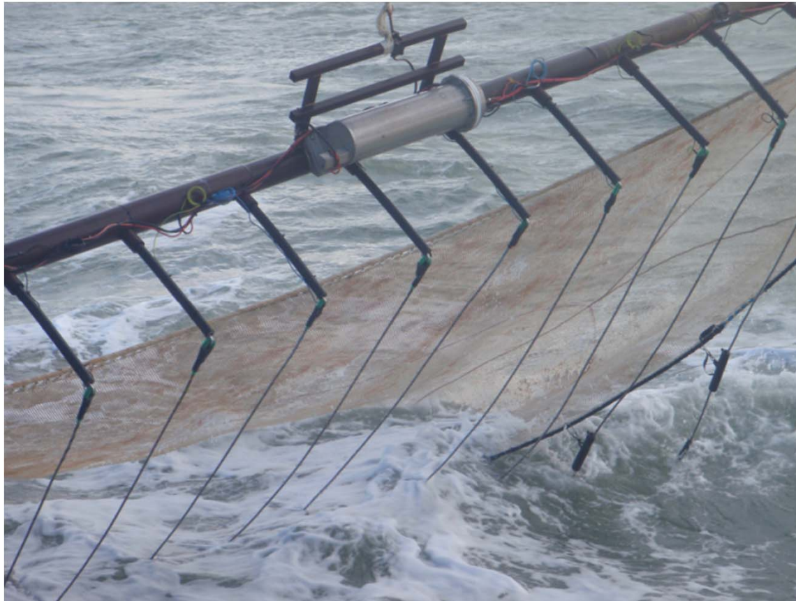
Brown shrimp ( Crangon crangon ) pulse trawl “Hovercran”(BE, NL)
