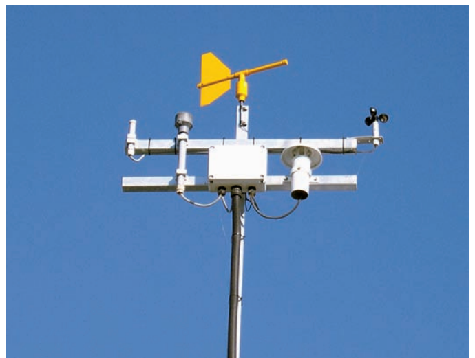
A meter for solar radiation (white, right/under), should not be shaded by other parts of the meteorological station.
