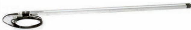
The best sensor for measuring light in a greenhouse is a Li-cor line quantum sensor (LI-191), that measures the average light intensity over 1 m length. Photo: www.licor.com
