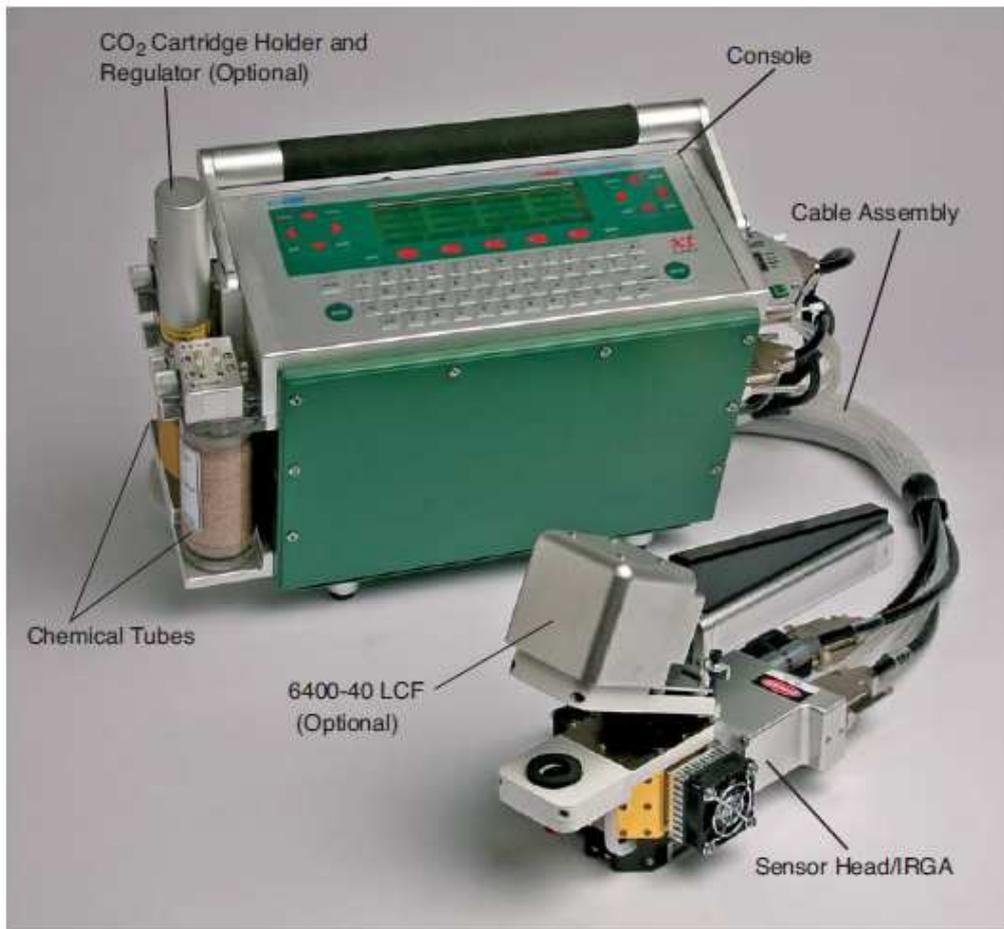
**Figure 2. LI-6400XT portable photosynthesis system (LI-COR Biosciences), picture taken from the manual of the LI-6400XT LI-COR, Inc. © Copyright 1998 - 2004, LI-COR, Inc.**
