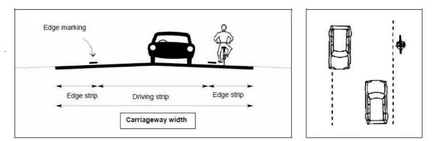
Figure 1. Minor rural access road type I as proposed by the SWOV Institute for Road Safety Research: driving strip with edge strips. Cross section (left) and view from above (right). Source: [9]
