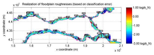
Figure 3. One of the 15 realizations with new floodplains roughnesses, based on the ecotope map purities (roughness variation at ecotope polygon level)
