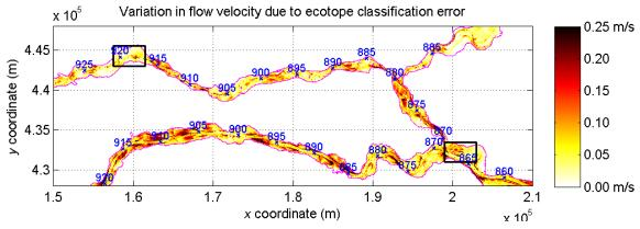
Figure 5. Local standard deviations in flow velocities, based on the 15 realizations of roughness maps (roughness variation at ecotope polygon level, based on map purities).
