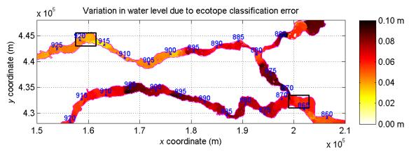
Figure 6. Local standard deviations in water levels, based on the 15 realizations of roughness maps (roughness variation at ecotope polygon level, based on map purities).
