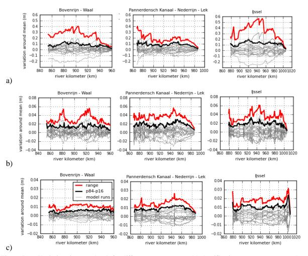
Figure 7. Variations in water levels for different error sources: (a) classification errors at ecotope polygon level, (b) classification error at computational cell level, and (c) within class variation. Note the different vertical axis between the a, b, and c.
