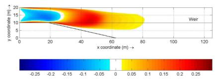
Figure 2 – Top view of sedimentation (red) and erosion (blue) [m] around a longitudinal weir
