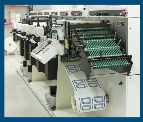
Printing machine specially equipped for printing organic electronics. With e,g.; flexo-printing, rotative screen, lamination, cutting etc, roll-to-roll 30 cm wide, 5 – 120 m/min printing speed.
