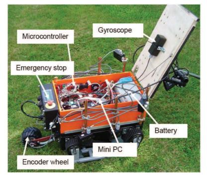
Figure 2: The components of Cropscout II (2)
