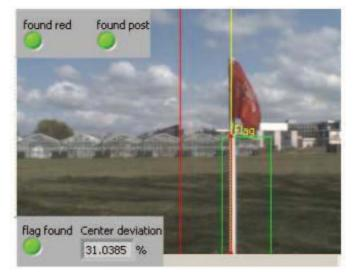
Figure 6: Locate position of corner flag by computer vision
