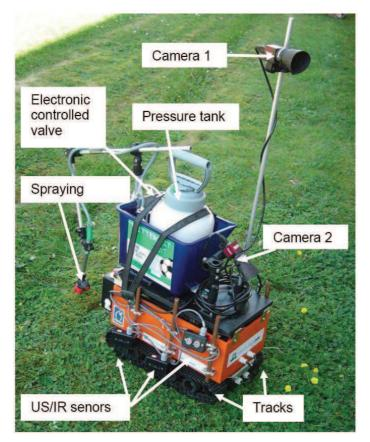
Figure 1: The components of Cropscout II (1)
