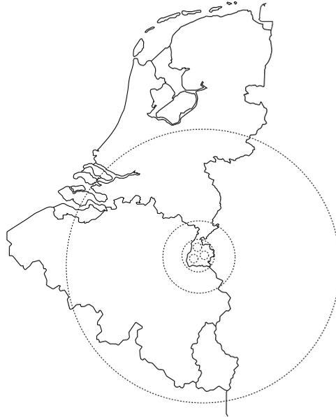
**Figure 3-7.** Transportation distances (from the centre to the outside) for energy carriers originating in South Limburg (The Netherlands). Warm water should be transported a maximum of 10 km; solid biomass a maximum of 50 km. Liquid fuels can be transported over longer distances depending on the mode of transportation. Electricity can be transmitted with a loss of approximately 10% over 1000 km.
