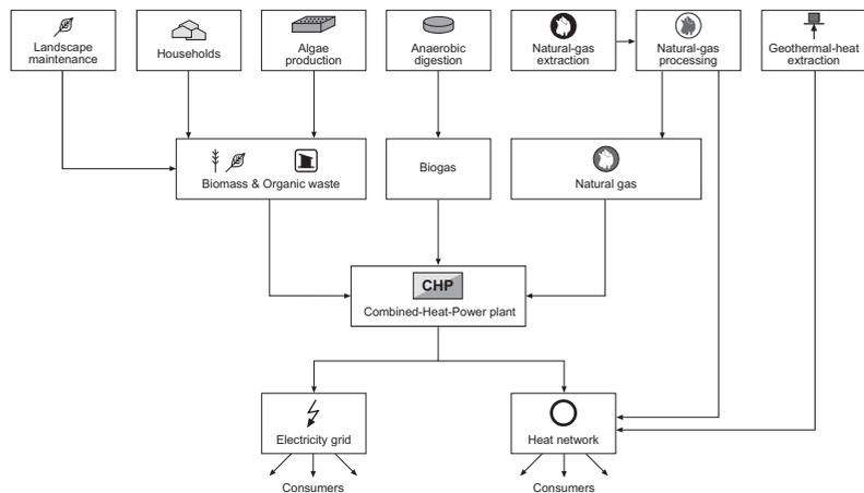
**Figure 6-3.** Interdependencies between the different energy system levels: energy carriers, conversion technologies, networks and consumers. Energy study for Southeast Drenthe.
