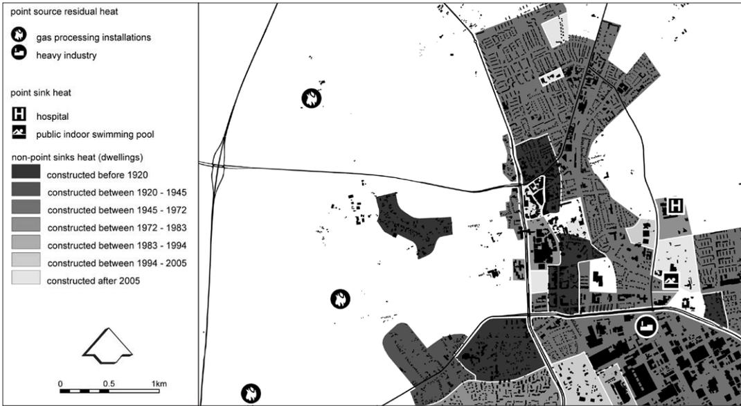
Figure 5-9. Residual heat sources and potential heat sinks in Emmen, The Netherlands.
