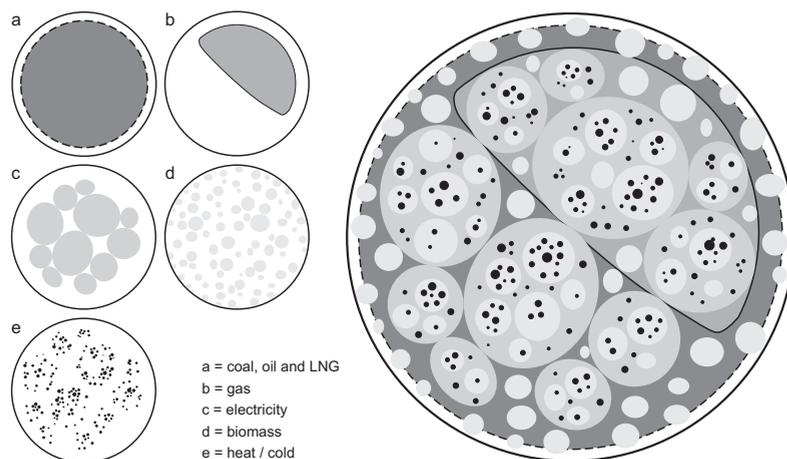
**Figure 6-2.** Different energy systems with relative system size. Coal, oil and LNG are distributed across the entire planet. Gas networks, on the contrary, extend only over certain parts of the planet. Electricity networks are again smaller but interconnect with each other. Second generation biomass is usually utilized within a region. Yet, heat/cold networks are smaller and extend over a neighbourhood or parts of a town.
