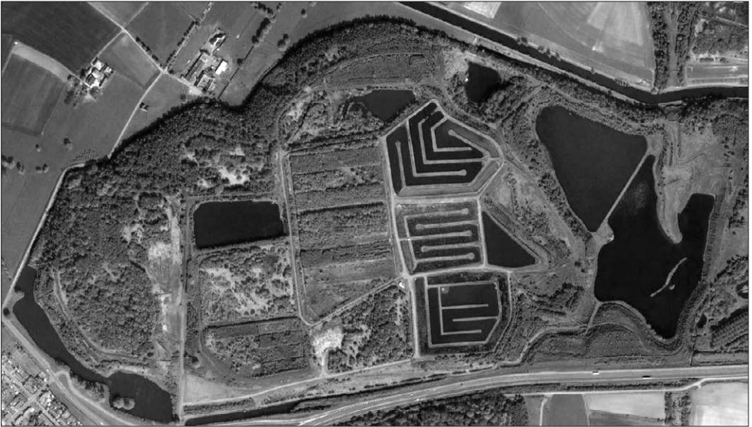
**Figure 3-5.** Aerial photograph of an ecological waste-water treatment plant in Lallaing (France) designed by H2O Mosaic. Scale approximately 1:10 000 (photograph Google Earth).
