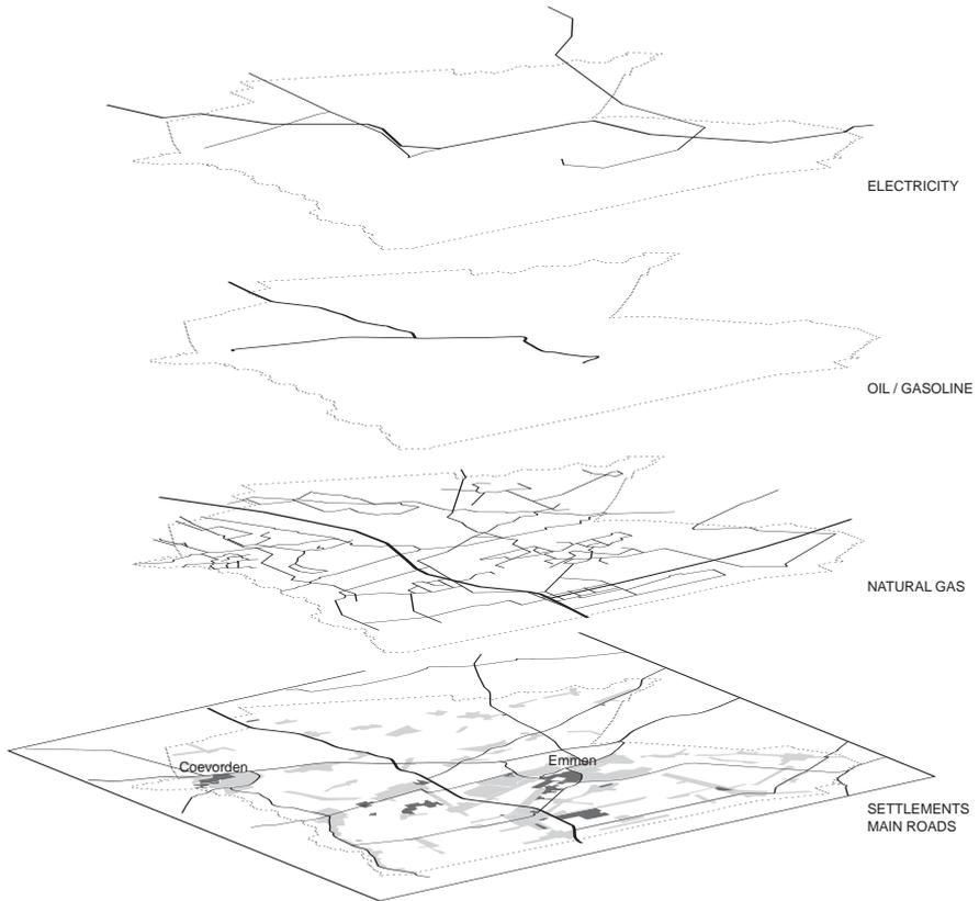
**Figure 6-6.** Different energy subsystems in the region of Southeast Drenthe.
