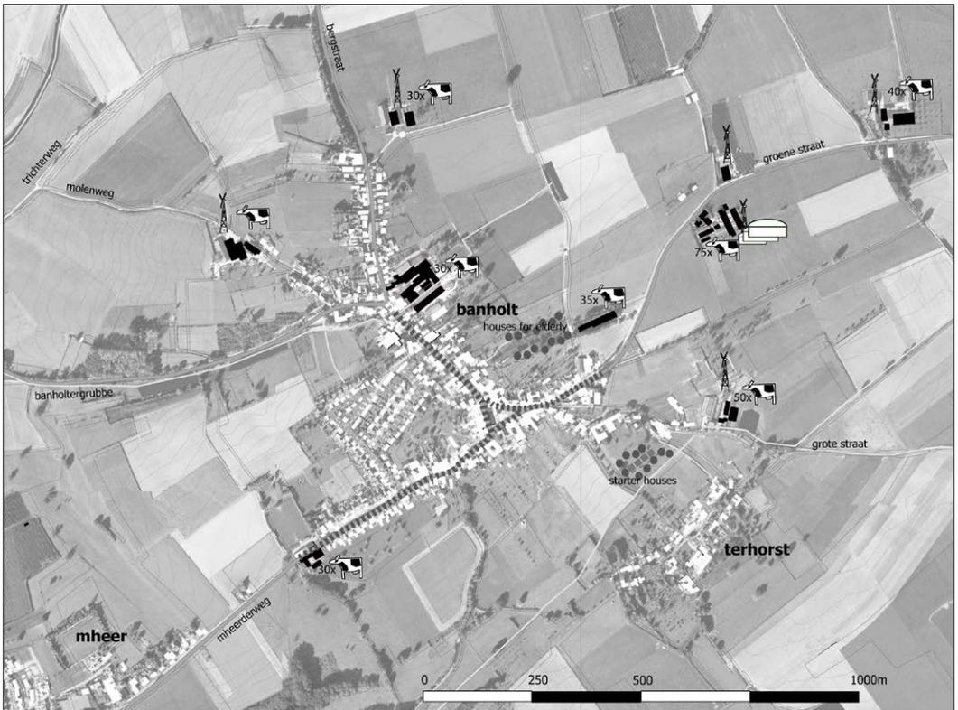
**Figure 3-11.** Potentials for synchronising energy demand and supply in the rural community of Banholt (The Netherlands). Manure from cattle rearing can be stored on individual farm plots (indicated in black) or directly processed into biogas at the central conversion plant (white symbol). Biogas can be stored or injected into the existing natural-gas grid (courtesy of K. Neven).
