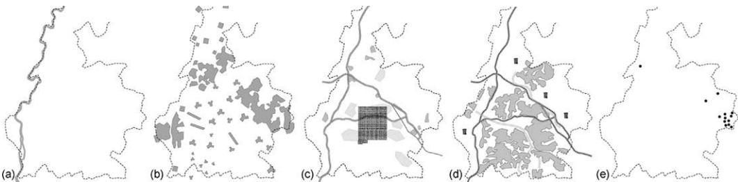
**Figure 3-9.** Quick-scan energy potential mapping at a regional scale in South Limburg (The Netherlands). Potential for (a) hydro power; (b) solar energy; (c) wind energy; (d) biomass; (e) geothermal energy.
