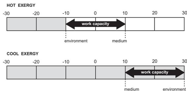
**Figure 4-1.** Comparison between hot and cool exergy. The work capacity of a medium with 10°C temperature at an environment temperature of -10°C is similar to a situation with 30°C in the environment.
