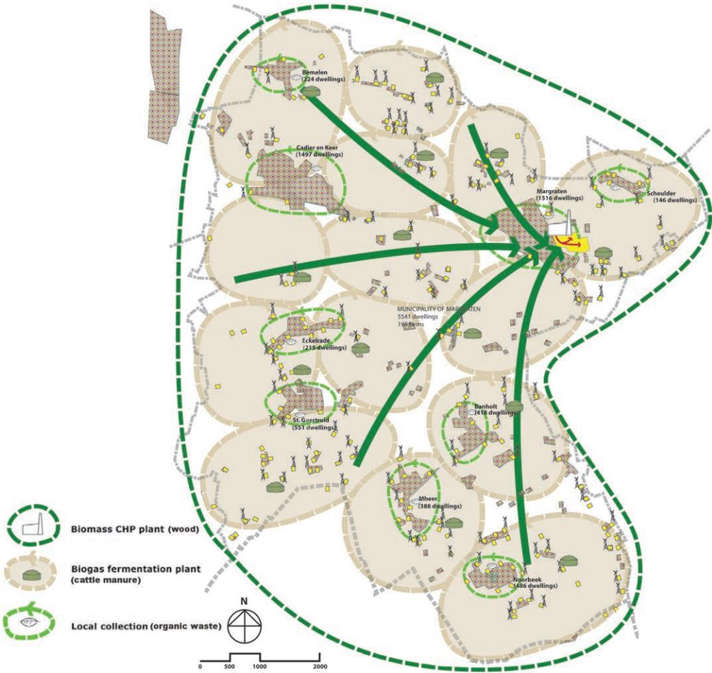
**Figure 5-7.** Proposal for differentiated energy subsystems in the municipality of Margraten (spatial extent indicated with dashed lines). A single CHP near the village of Margraten processes woody biomass from the entire municipality. Decentralized biogas fermentation plants in the different villages process local manure and organic household waste.
