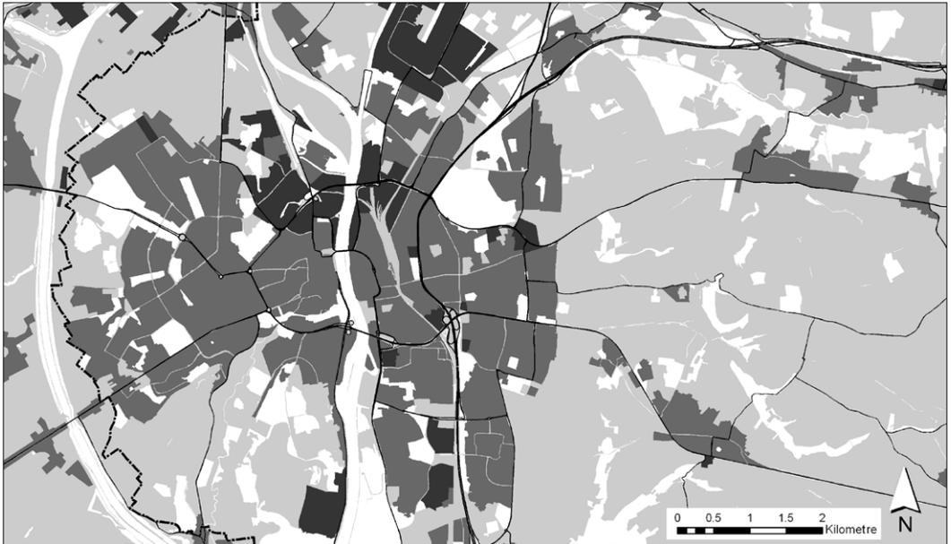
**Figure 3-2.** Potential locations for the assimilation of solar energy in the Maastricht area in the Netherlands. Dark grey indicates industrial areas and business parks, with high potential due to flat roofs. Mid-grey indicates residential areas where there is moderate potential. Light grey indicates open land where the potential is low. Pale grey areas are water, forest, and nature areas with restrictions for energy assimilation.
