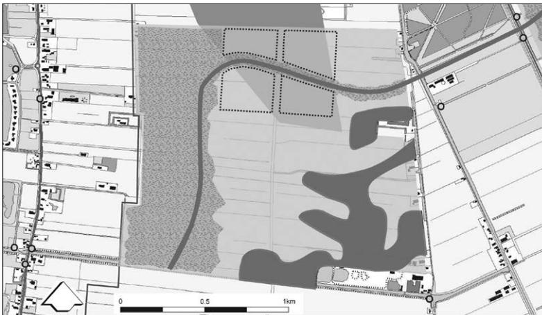
**Figure 3-8.** Construction of new neighbourhoods (indicated by a dashed line) above an aquifer (dark grey) providing warm water for room heating. Energy-potential study Hoogezand-Soetermeer (The Netherlands).
