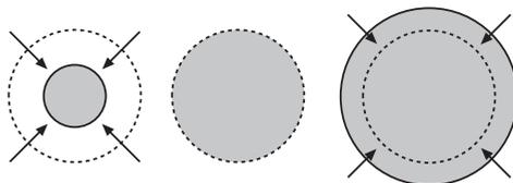
**Figure 3-6.** Deviation from optimum system size (indicated by dashed line) necessitates additional energy subsidies (arrows). The size of the left-hand system is smaller than its energetic optimum; the right-hand system is larger than its optimum system size.
