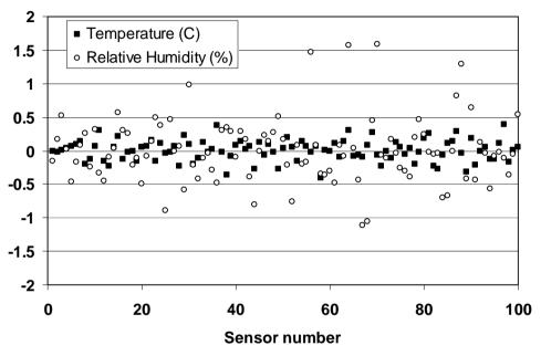
Observed deviations:  $\pm 0.4 \, ^{\circ}\text{C}$  and  $\pm 1.5\%$  (within spec). Check and adjust offset by producer. Use sensor element with higher spec ( $\pm 0.3 \, ^{\circ}\text{C}$ )
