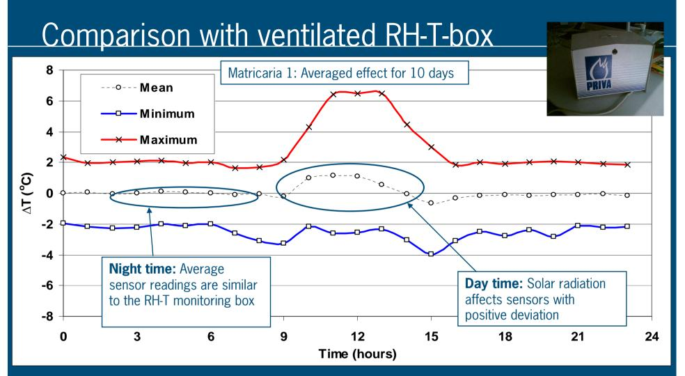
Advice to producers: Use ventilated boxes or a well-designed radiation shield.
