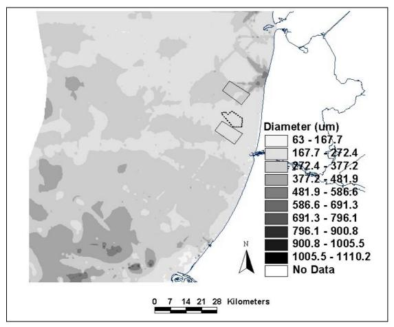
**Figure 4.** Grain size of the sediment (diameter in µm) in the Dutch coastal zone. The dotted line indicates the planned area of the wind farm, the solid squares indicate reference areas. GIS data from the Flyland project (2001).
