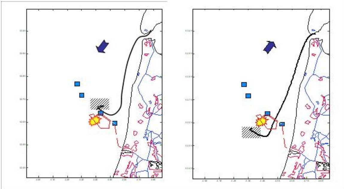
**Figure 3.** Possible transits (black line) to an anchoring position (hatched area) near the pile driving site (star), at different wind directions, indicated by blue arrow. Offshore gas production platforms in the area are marked (blue blocks) as is a gas pipeline connecting the two nearshore platforms to the mainland (red line); these structures had to be avoided for safety (collision, anchoring) and operational (blocking the view) reasons.
