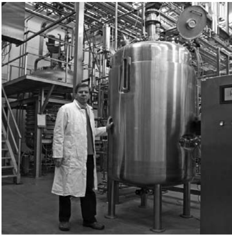
Figure 3.1. Mass-production equipment (left: 1000 litre fermentor for liquid state fermentation; right: 1.3 m 3 bioreactor for solid state fermentation)
