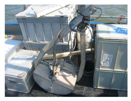
Figure 2 Van Veen grab used to ground truth the seabed (0.1  $m^2$ ).
