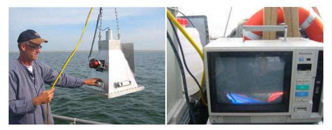
Figure 1 a: The "water lens" video system as developed by TNO-IMARES. A light is attached to the side. Visible are the wing and the bars of led. b: the monitor on deck.
