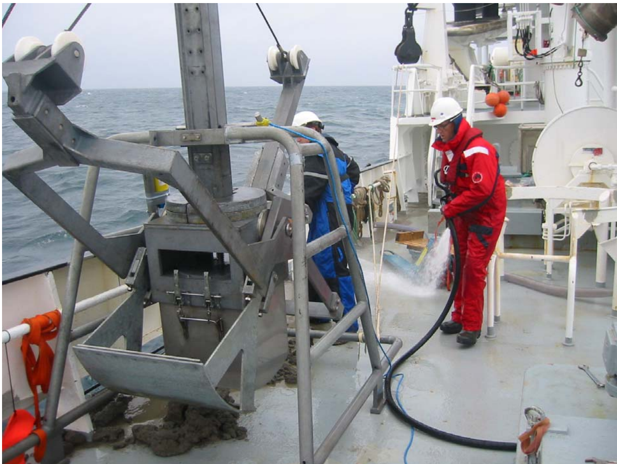
Figure 3: Haja box corer used at the Aberlour prospect
