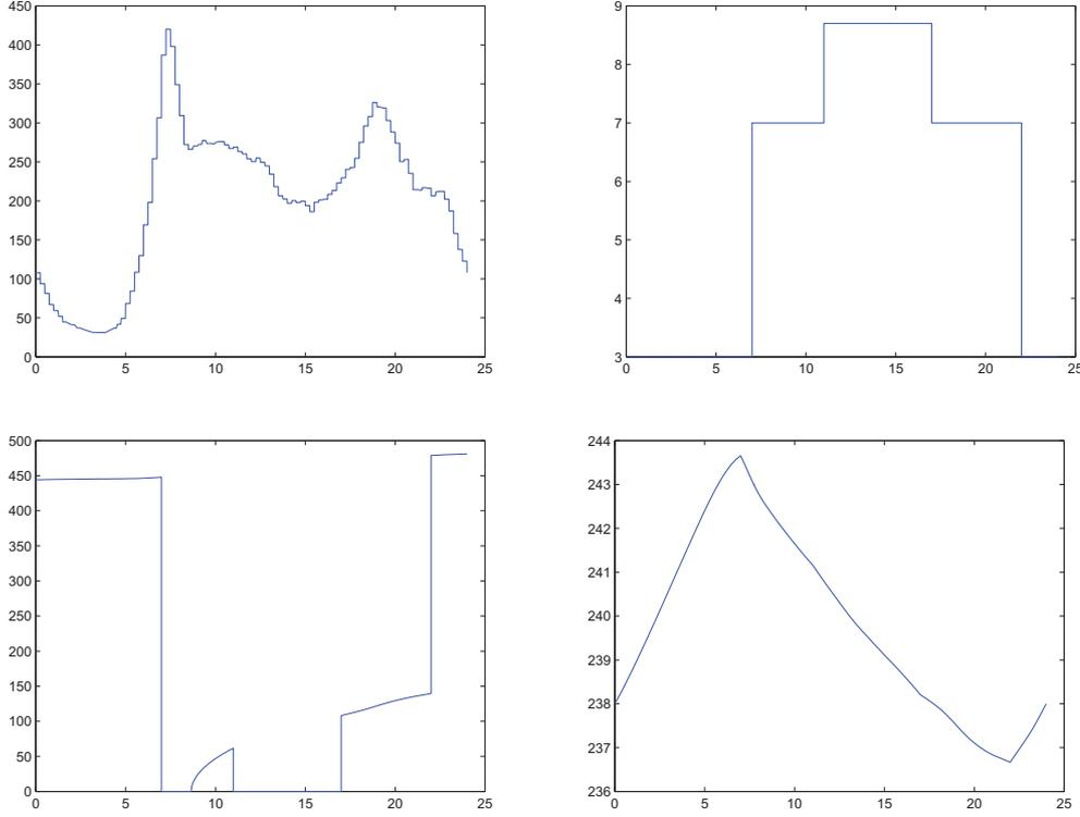
Figure 6.5: Upper left: Water demand  $F_{\text{out}}$  in Smithville. Upper right: Energy costs  $c(t)$  per kWh. Bottom left: Optimal water flow  $u = F_{\text{in}}$  through pumps. Bottom right: Reservoir level  $x = L_{\text{res}}$  in case of optimal flow.
