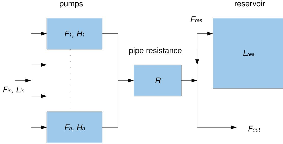
Figure 6.4: A module consisting of a set of  $n$  water pumps, a pipe with resistance  $R$  and a reservoir.
