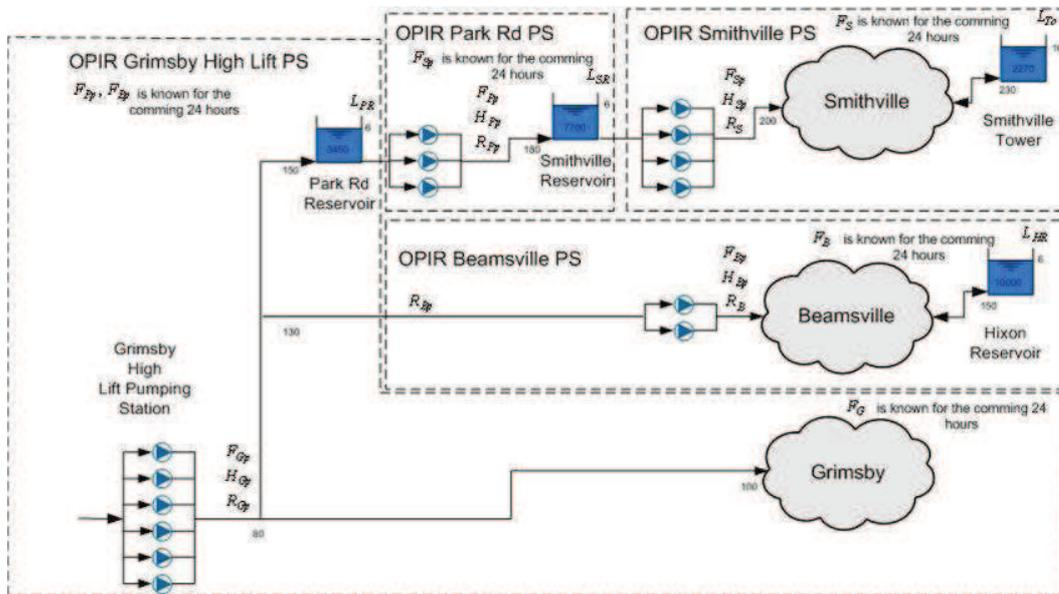
Figure 6.1: A sketch of the Grimsby drinking water supply region with the three towns Smithville, Beamsville and Grimsby, and the pump stations and the reservoirs.
