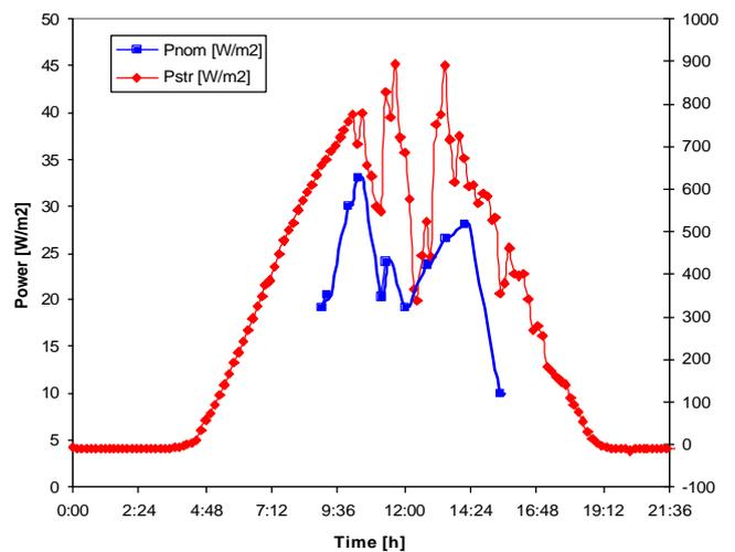
Figure 11 Generated electric power (Pnom) and incident radiation (Prad) on the location Wageningen measured on July. 31. 2008
