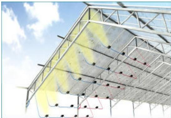
Figure 1: Impression of a greenhouse hood with normal Fresnellenzen integrated between double glass (Drawing Bode Project and Engineering).
