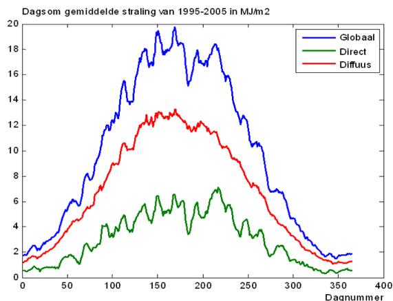
Figure 2 Daily average global radiation in the Netherlands divided into diffuse and direct part.
