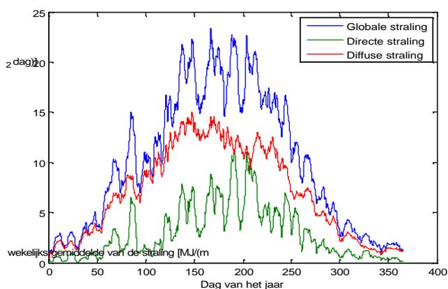
Figure 11 Daily radiation sums (global, direct and diffuse part) for a year measured in De Bilt.
