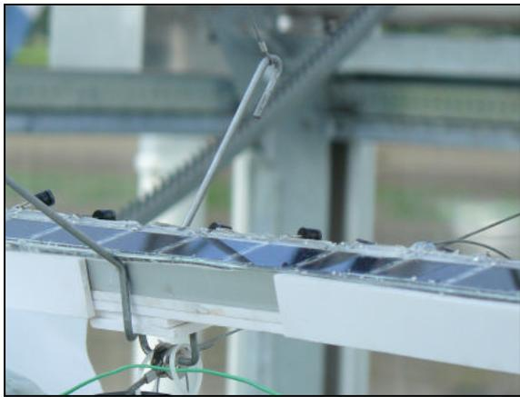
Figure 8 The TPV module of the system with the silicon cells inside the greenhouse
