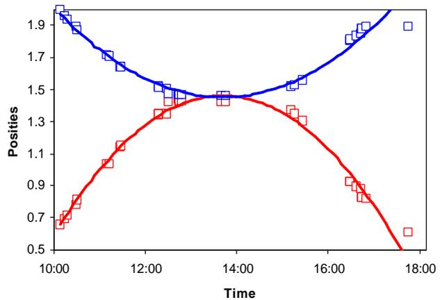
Figure 10 Both positions of the electric motors where the module will be held in the focus on August 15, 2008. R1 is the position of motor which regulate the vertical movement and R2 is the position of the motor which contribute to the horizontal movement.
