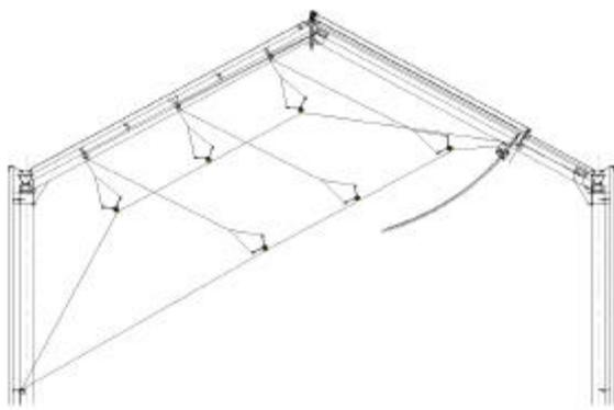
Figure 9 Cross section of the hood with details of the suspension and steering construction of the solar cell modules, with the lowest and highest position of the modules is shown.
