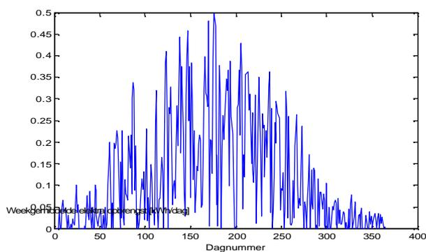
Figure 12 Week average of the electrical power output as a function of the day number.
