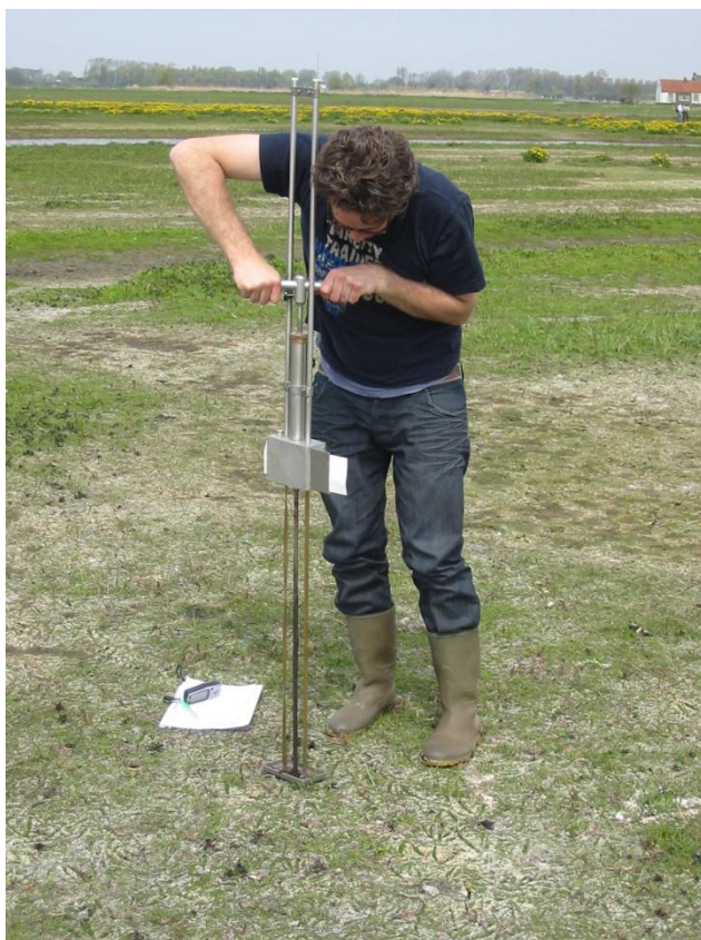
Foto 6 Zelfregistrerende penetrograaf, meting in Kogjespolder, Overstromingsgrasland.
